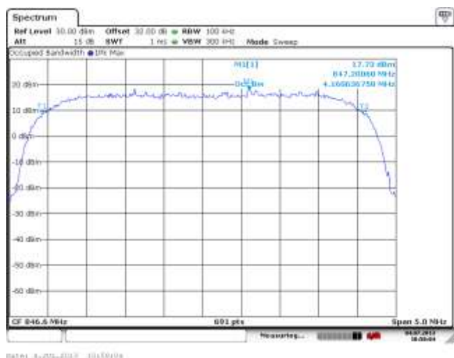
Figure 2-15a: Occupied Bandwidth, Band 5 High Channel
