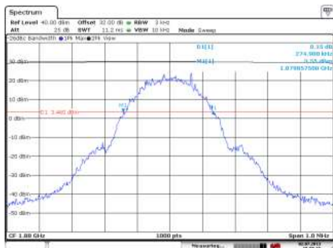
Figure 1-21a: -26dBc bandwidth, PCS1900 Middle Channel in GSM mode
