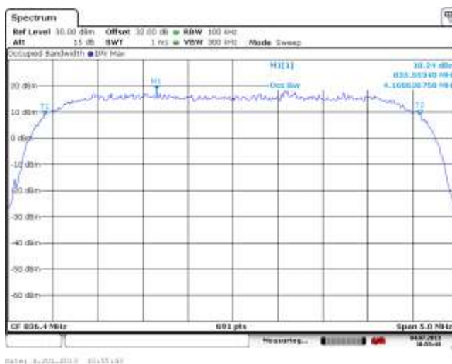
Figure 2-14a: Occupied Bandwidth, Band 5 Middle Channel
