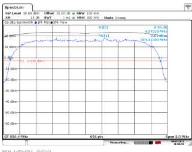
Figure 2-19a: -26 dBc Bandwidth, Band 5 Low Channel
