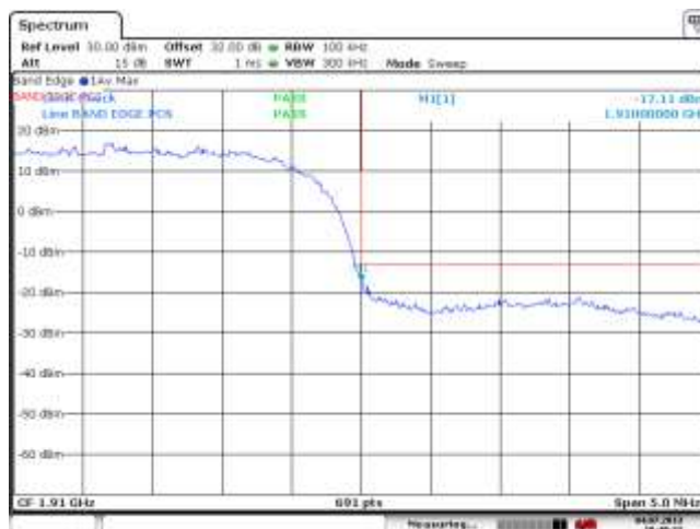
Figure 2-28a: Band 2 High Channel Mask
