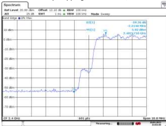
Figure 4-41: Band Edge Compliance Freq. Hopping, Static PBRs, 2-DH5
