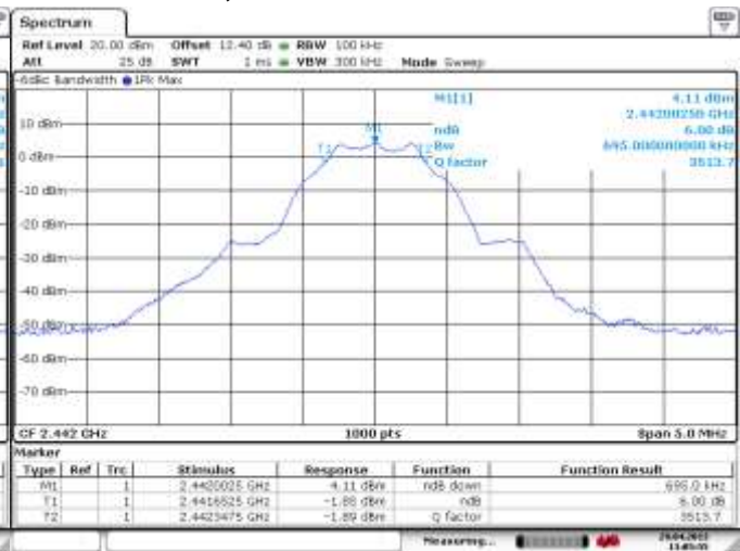
Figure 4-60: 6 dB Bandwidth LE, Channel 20
