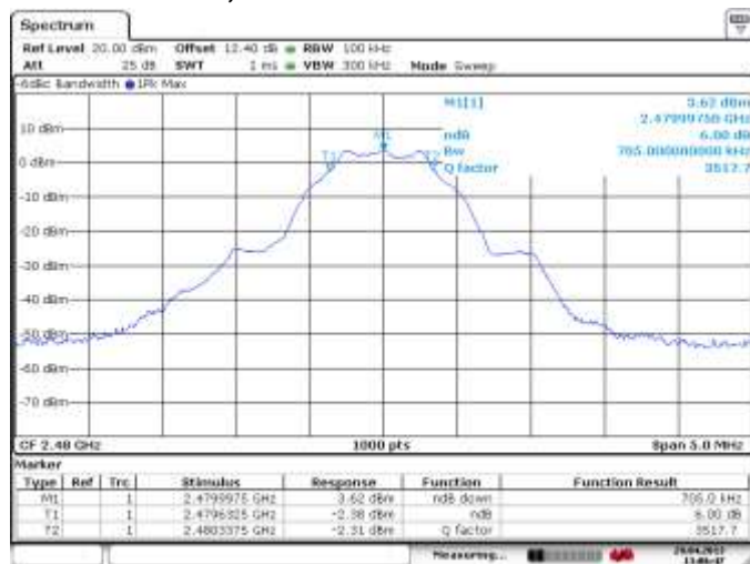
Figure 4-61: 6 dB Bandwidth LE, Channel 39
