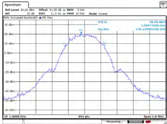
Figure 1-37a: Occupied Bandwidth, PCS1900 Band, High Channel in EDGE mode
