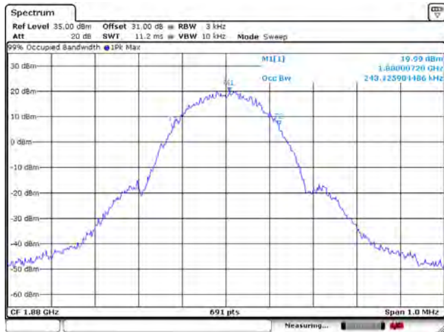
Figure 1-36a: Occupied Bandwidth, PCS1900 Band, Middle Channel in EDGE mode
