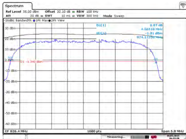
Figure 1-19b: -26 dBc Bandwidth, Band 5 Low Channel
