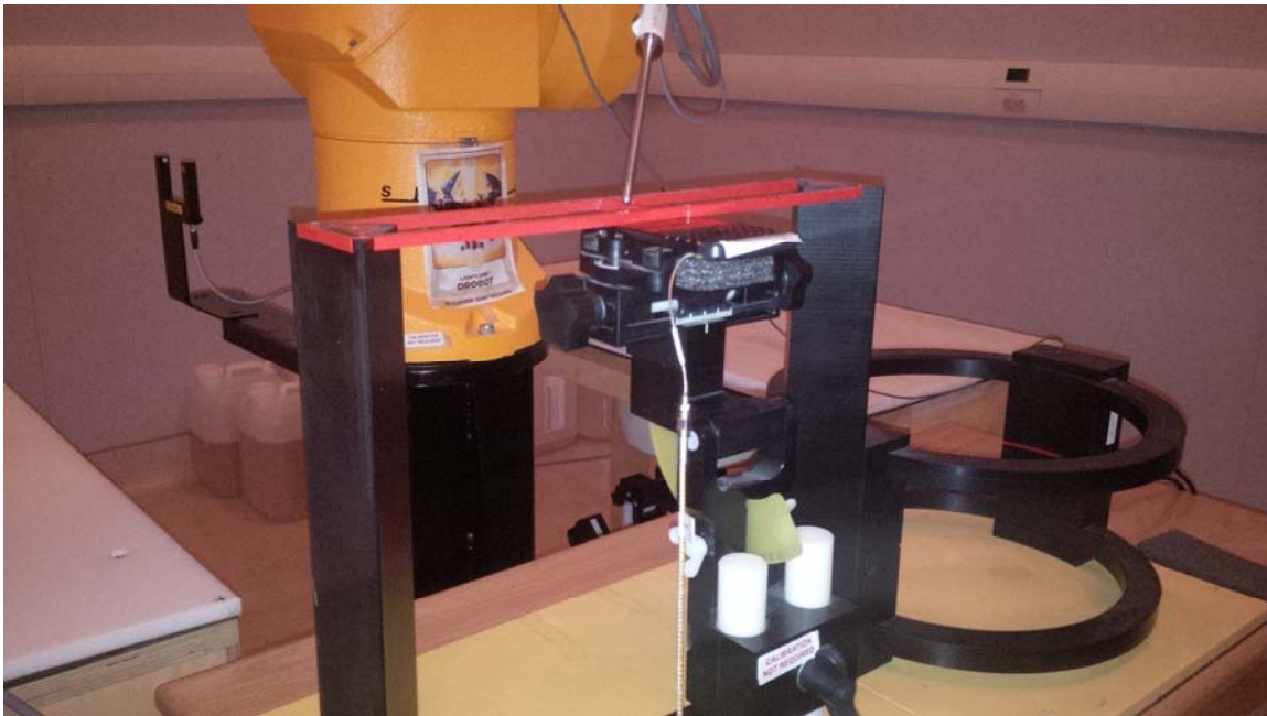
Figure E3: Audio Band Magnetic (ABM) T-Coil measurement setup
