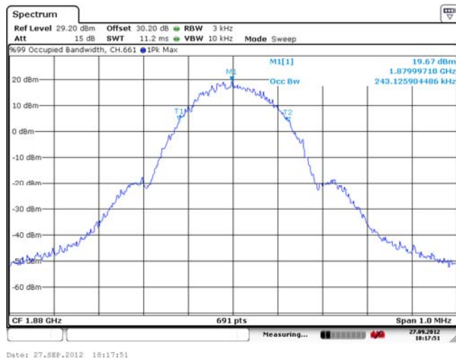
Figure 1-33a: Occupied Bandwidth, PCS1900 Band, Middle Channel in EDGE mode
