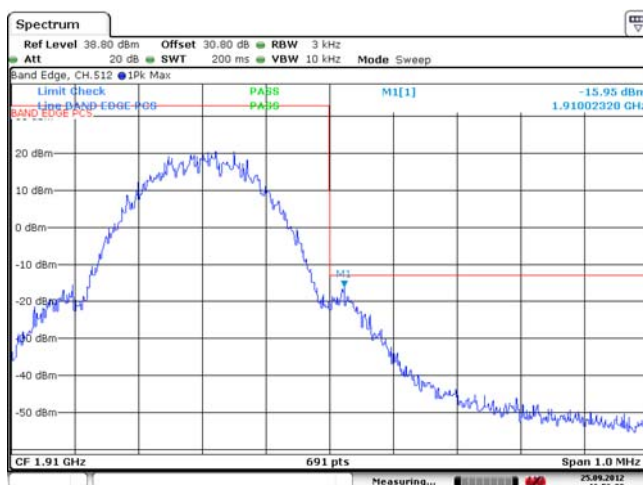
Figure 1-28a: PCS1900, High Channel Mask in GSM mode
