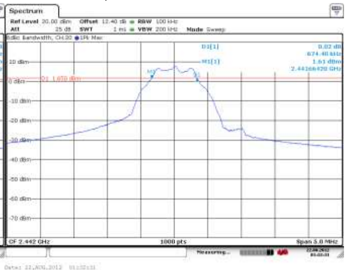
Figure 1-60: 6 dB Bandwidth LE, Channel 20
