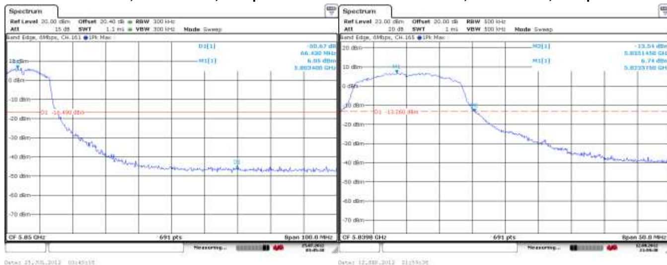
Figure 3-19: Band Edge Compliance 802.11a, Channel 161, 6 Mbps
