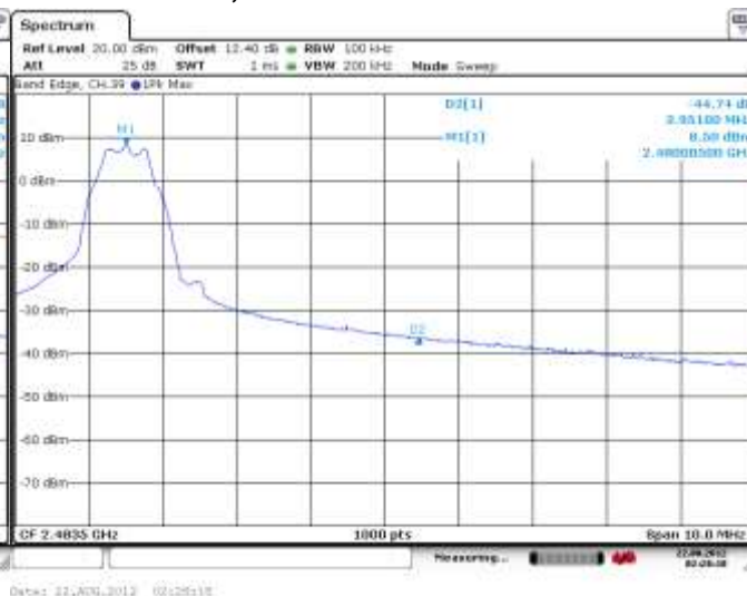
Figure 1-63: Band Edge Compliance LE, Channel 39
