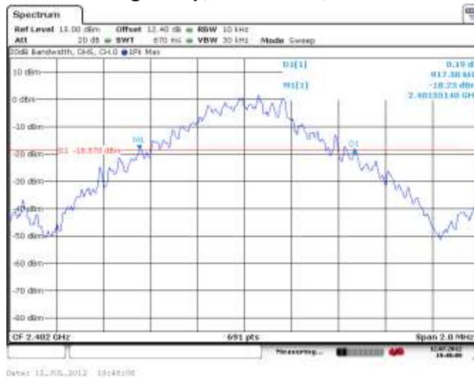
Figure 1-1: 20 dB Bandwidth Single freq., Static PBRs, DH5
