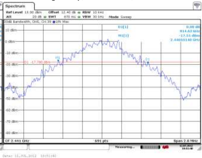
Figure 1-2: 20 dB Bandwidth Single freq., Static PBRs, DH5
