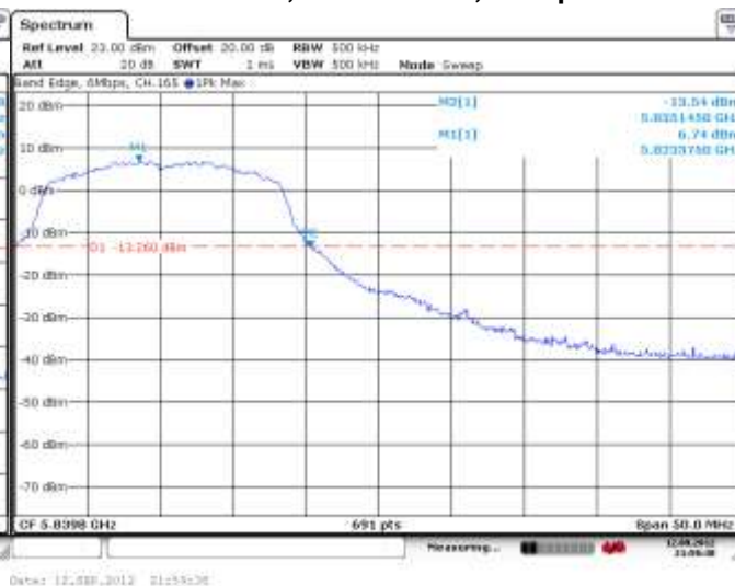
Figure 3-20: Band Edge Compliance 802.11a, Channel 165, 6 Mbps
