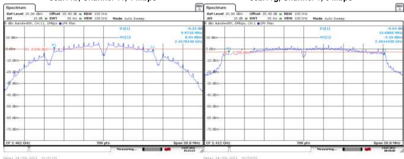
Figure 2-3: 6 dB Bandwidth 802.11b, Channel 11, 1 Mbps
