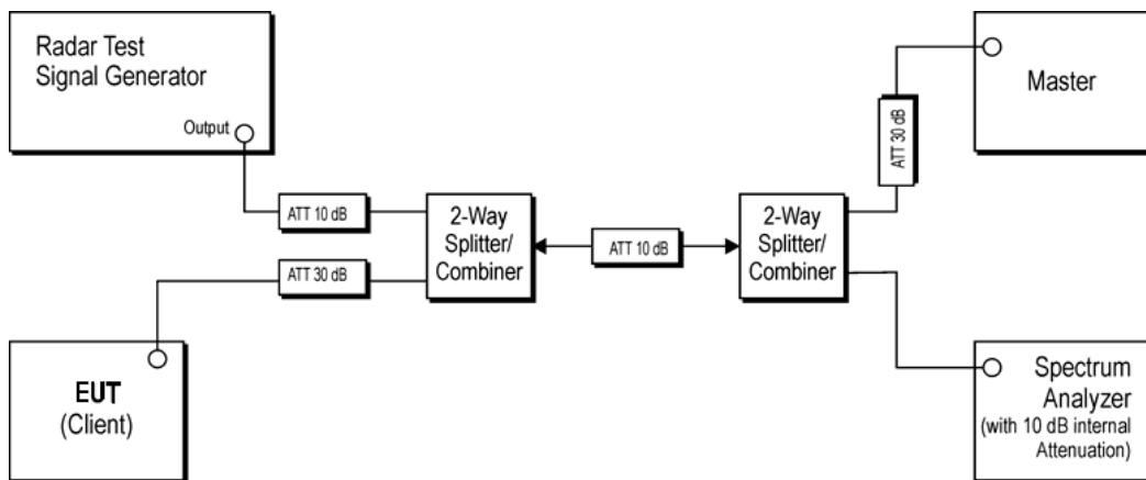
A spectrum analyzer is used as a monitor to verify that the EUT has vacated the Channel within the Channel Closing Transmission Time and Channel Move Time, and does not transmit on a Channel during the Non-Occupancy Period after the detection and Channel Move. It is also used to monitor EUT transmissions during the Channel Availability Check Time.
