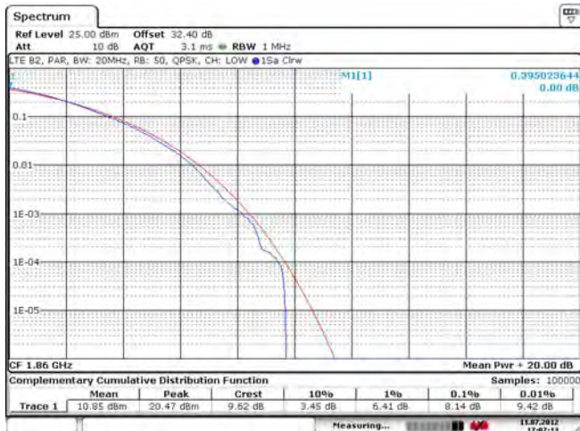
Figure 1-33c: Band 2 Low Channel PAR, 20 MHz BW, RB = 50
