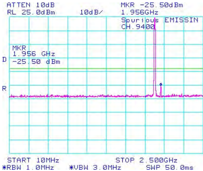
Figure 1-9b: BAND 2, Spurious Conducted Emissions, Middle Channel
