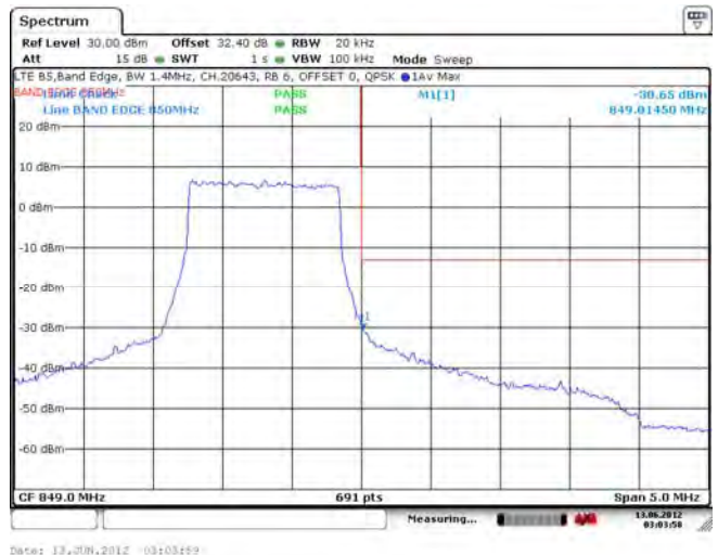
Figure 1-40d: Band 5 High Channel Mask, 1.4MHz BW, RB=6
