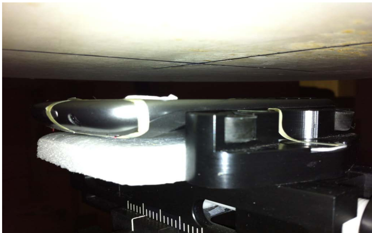
Figure E7. Body-worn configuration (No Holster, front side 15mm away)
