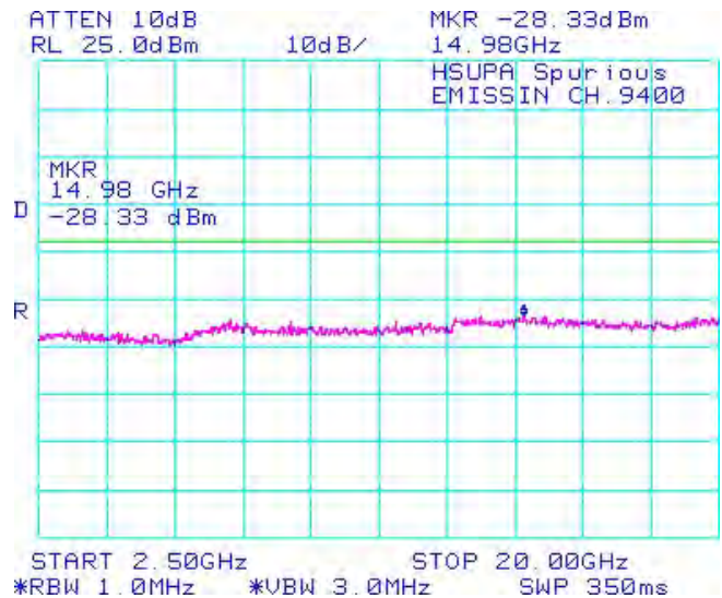
Figure 1-38b: Band 2, Spurious Conducted Emissions, Middle Channel
