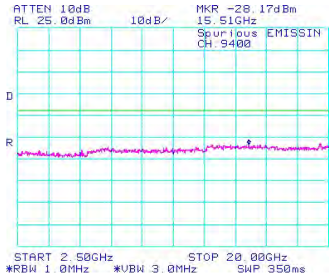
Figure 1-10b: Band 2, Spurious Conducted Emissions, Middle Channel
