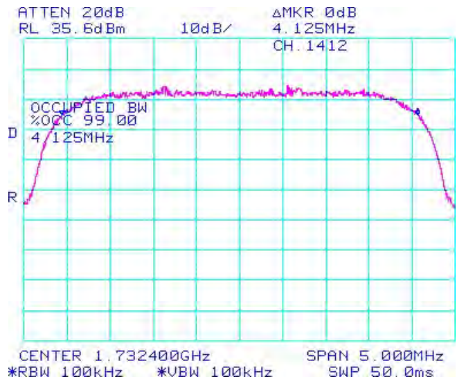
Figure 1-14b: Occupied Bandwidth, Band 4 Middle Channel
