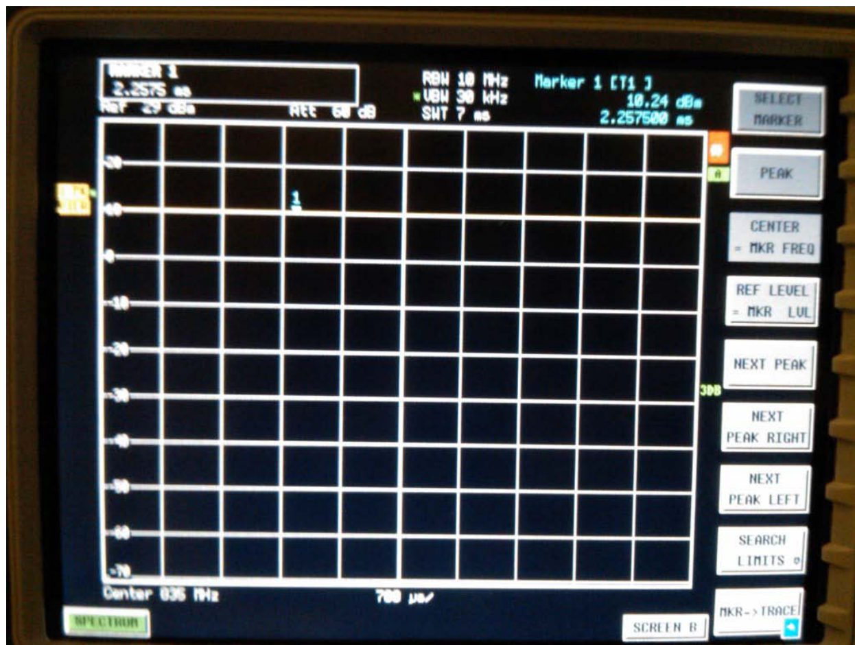
0 Hz Span CW Plot (835MHz)
