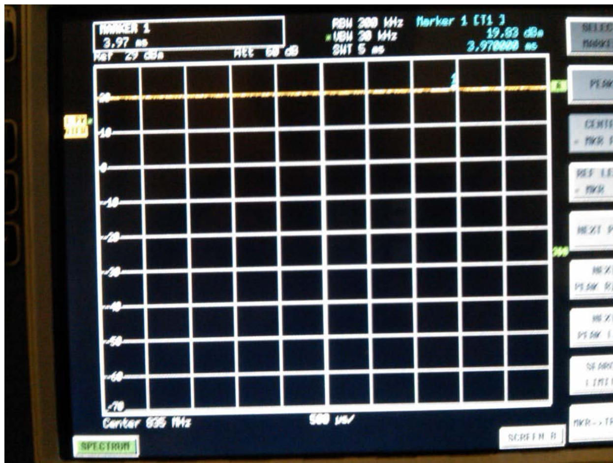
0 Hz Span CDMA Plot (835MHz)
