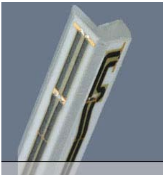
E-Field Probe (ER3DV6)
