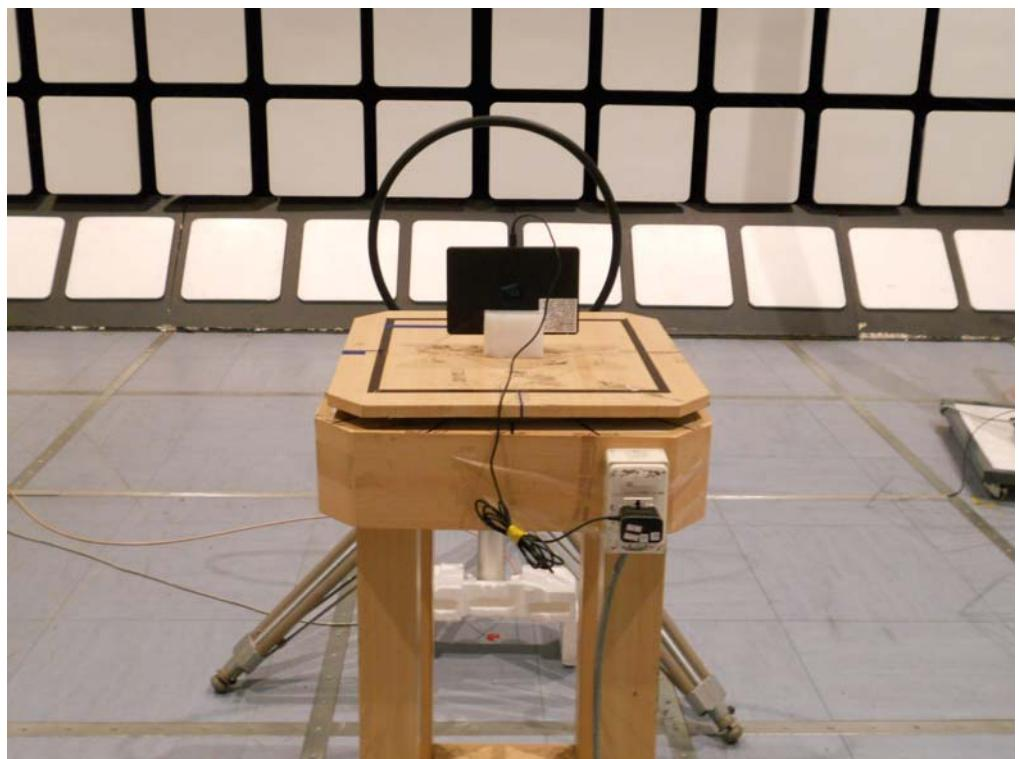
For radiated emissions 9kHz~30MHz
