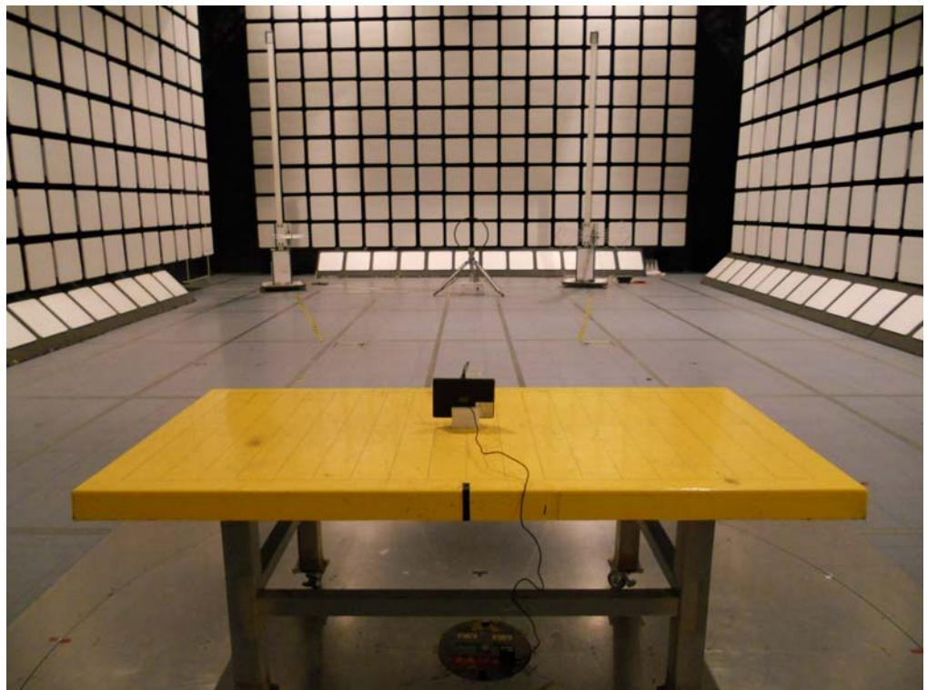
For radiated emissions 30MHz~1GHz
