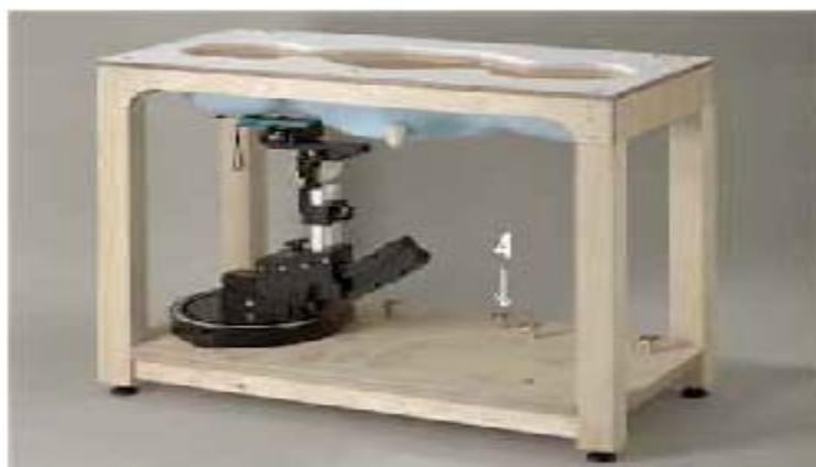
Figure 5.0.1. SAM Twin Phantom
