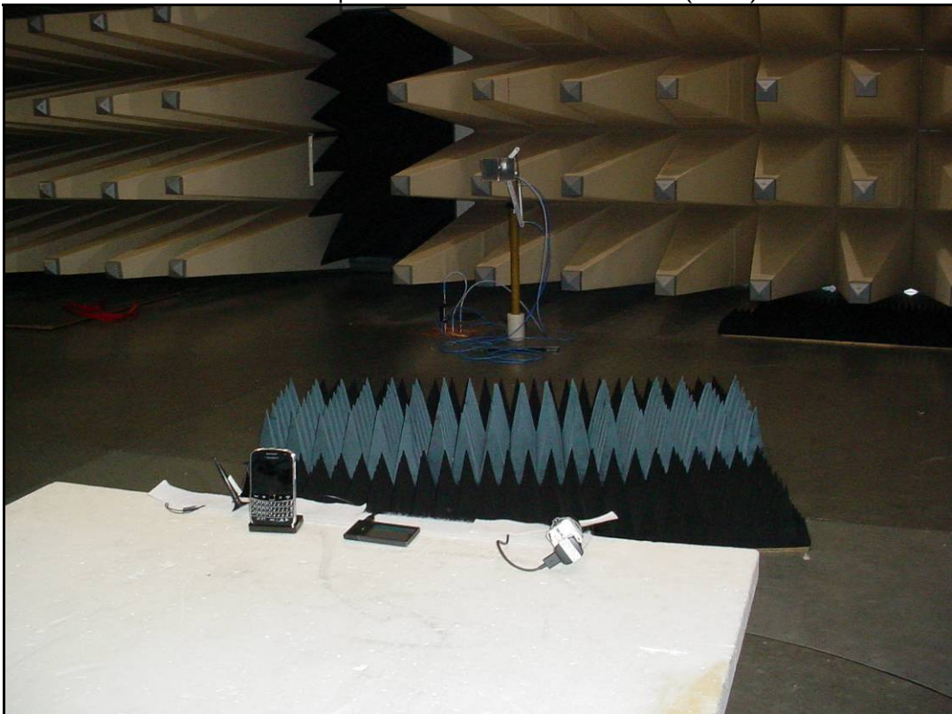
Photo 4: setup of radiated emission 1-10 GHz (set. 3)
