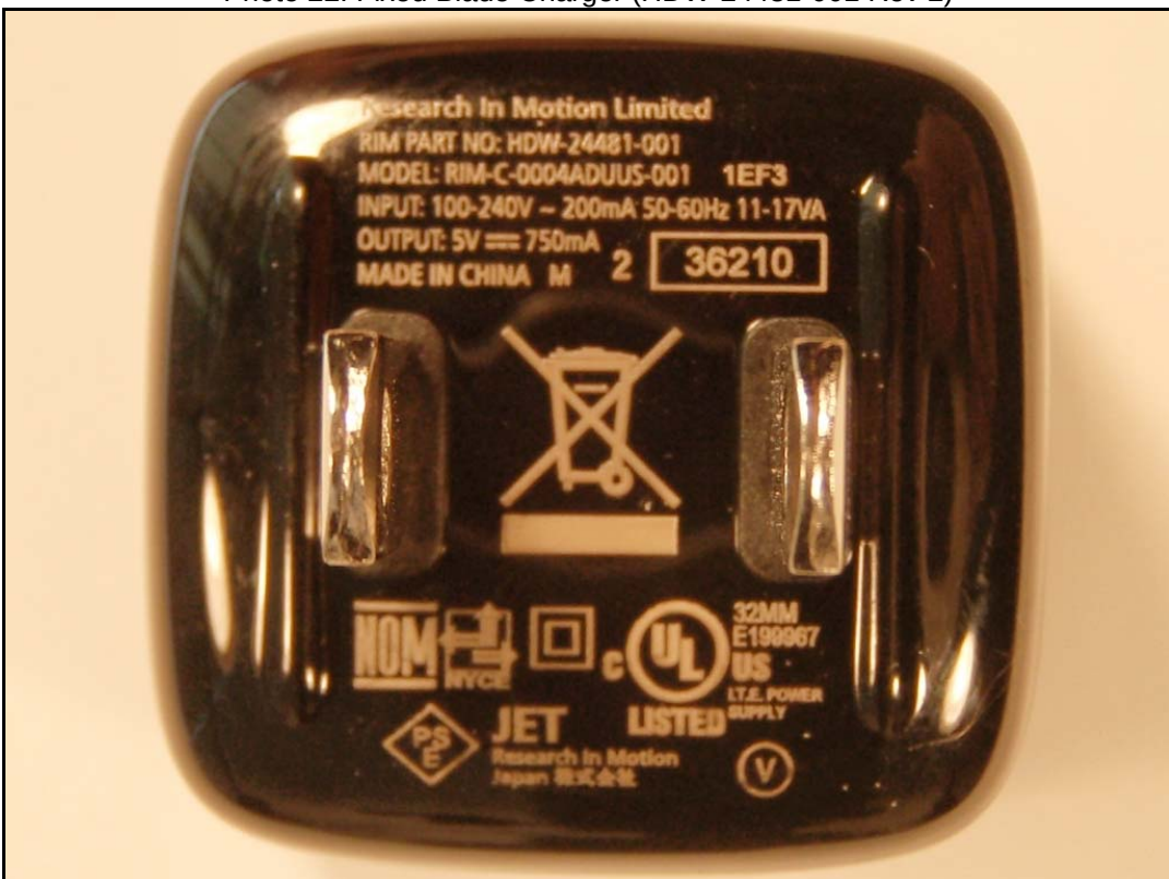
Photo 22: Fixed Blade Charger (HDW-24481-001 Rev 2)
