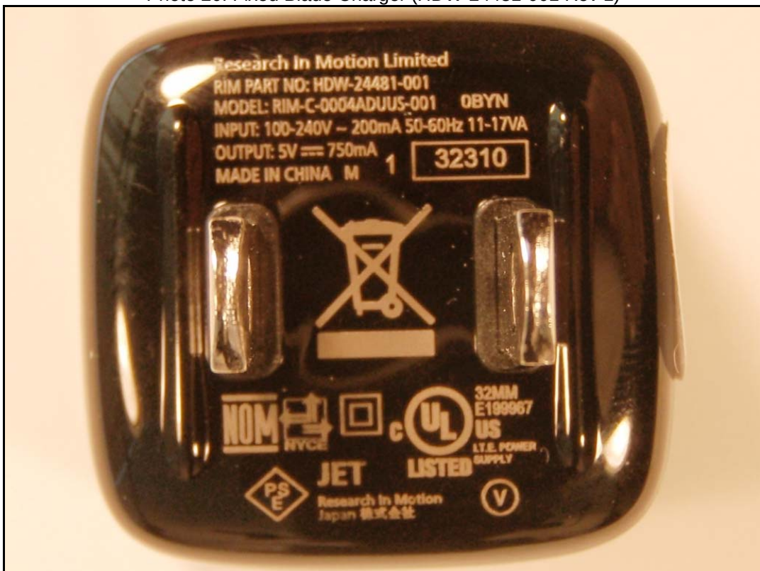
Photo 20: Fixed Blade Charger (HDW-24481-001 Rev 1)
