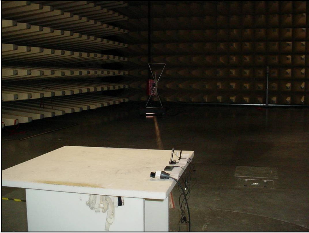
Photo 4: setup of radiated emission 1-10 GHz (set. 3)
