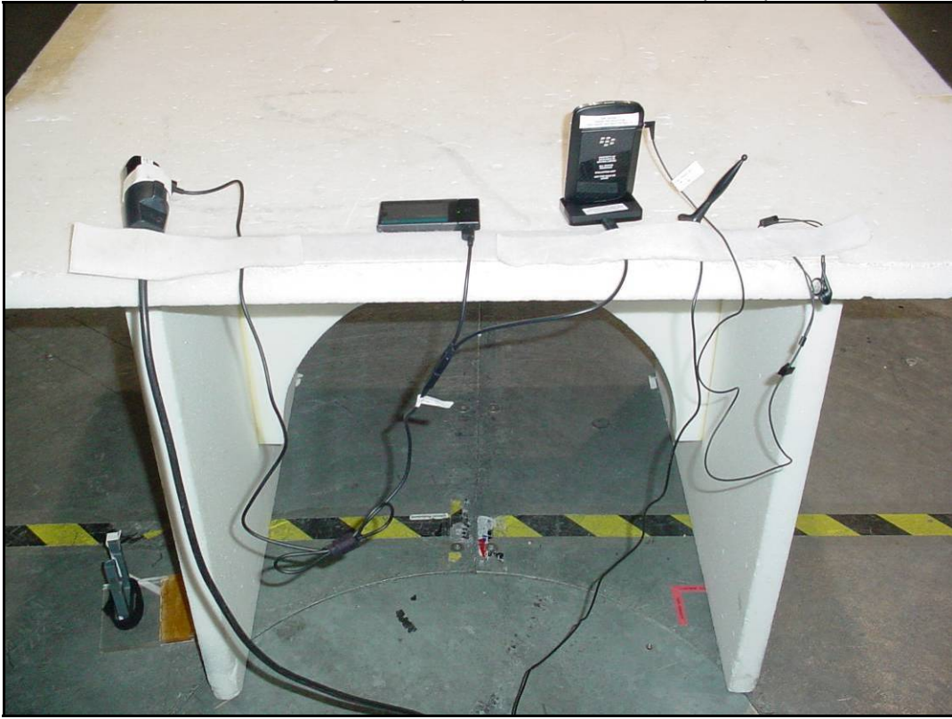
Photo 6: setup of radiated emission < 1 GHz (set. 4)
