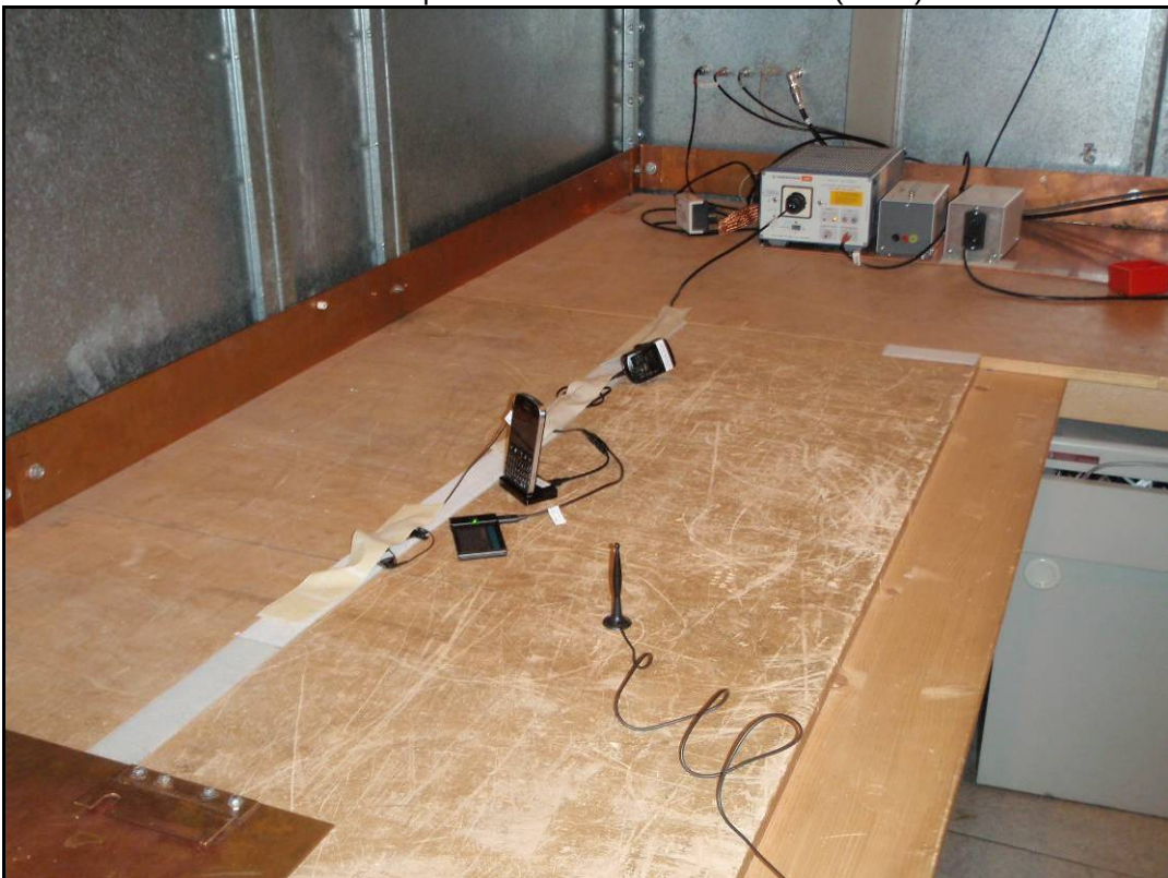
Photo 2: setup of conducted emission on AC (set. 2)
