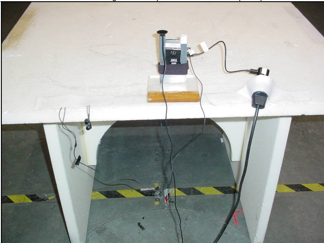
Photo 8: wiring of the setup of radiated emission (set. 4)
