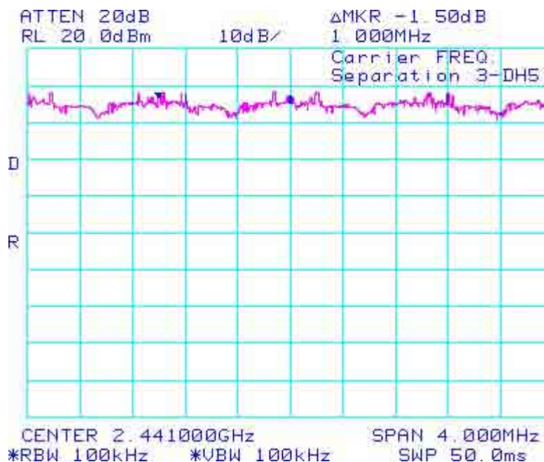
Figure 3-8: Carrier Frequency Separation, Freq. Hopping, Static PBRs, 3-DH5, Channels 38 to 39
