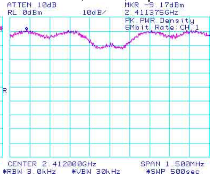
Figure 4-17: Peak Power Spectral Density
