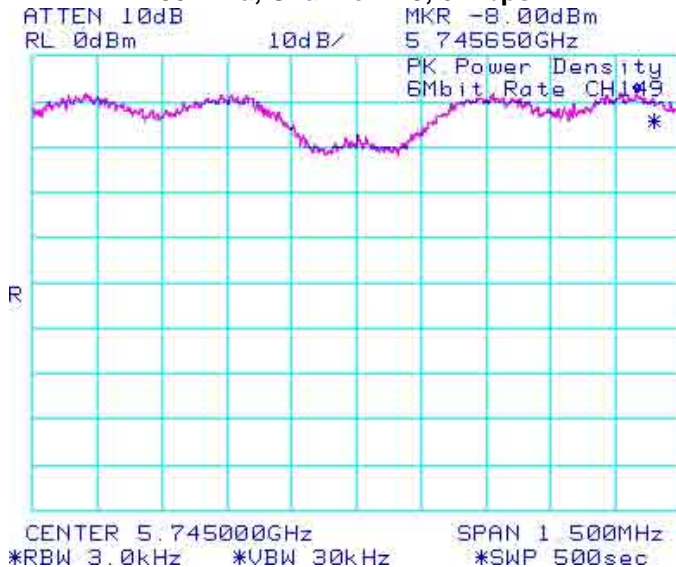
Figure 5-22: Peak Power Spectral Density
