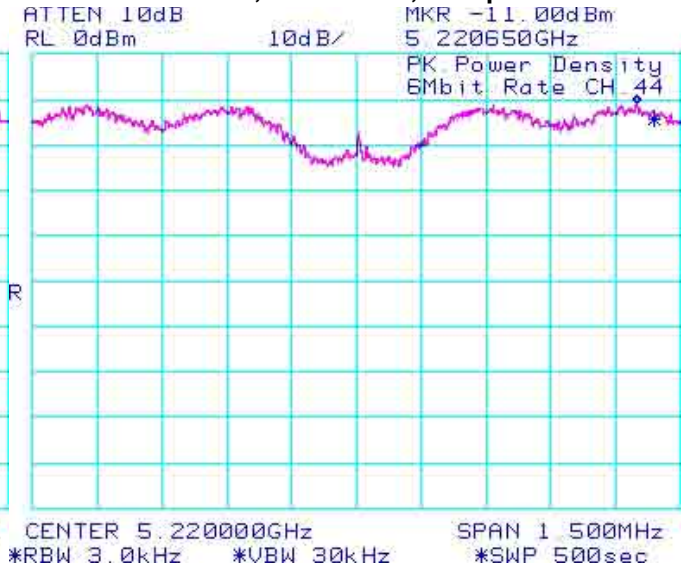
Figure 5-17: Peak Power Spectral Density 802.11a, Channel 44, 6 Mbps
