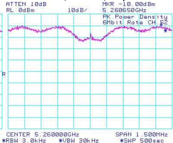
Figure 5-19: Peak Power Spectral Density 802.11a, Channel 52, 6 Mbps
