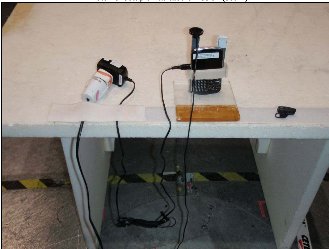
Photo 18: setup of radiated emission (set. 4)
