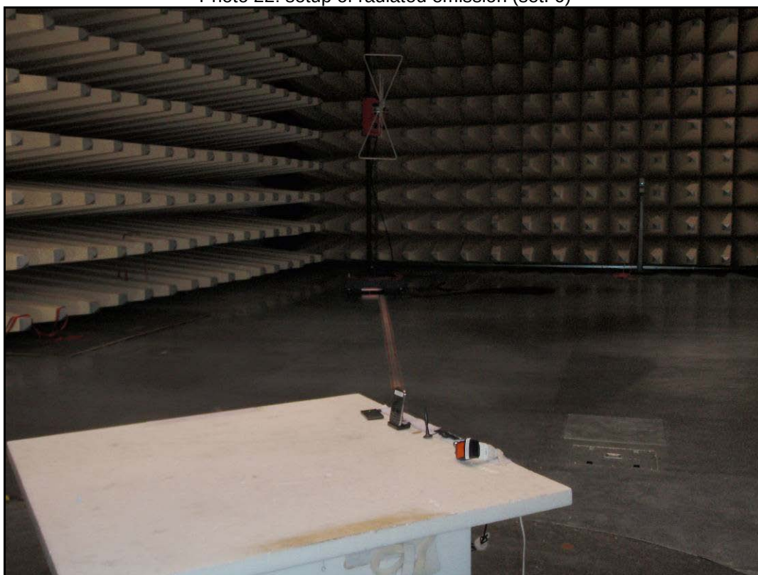
Photo 22: setup of radiated emission (set. 6)
