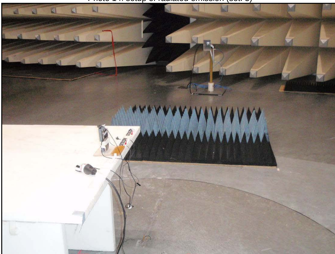
Photo 14: setup of radiated emission (set. 3)
