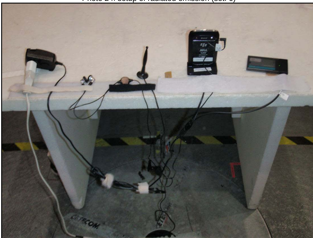
Photo 24: setup of radiated emission (set. 6)
