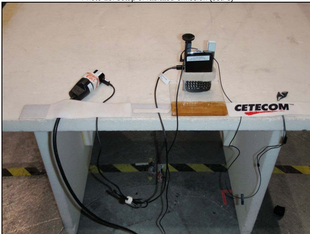
Photo 16: setup of radiated emission (set. 4)
