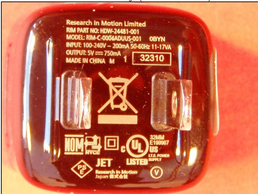
Photo 40: Fixed Blade Charger (HDW-24481-001 Rev 1)
