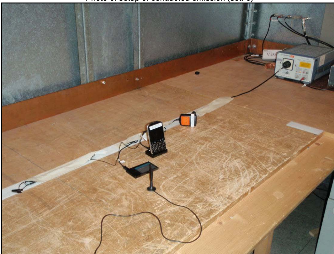
Photo 6: setup of conducted emission (set. 6)
