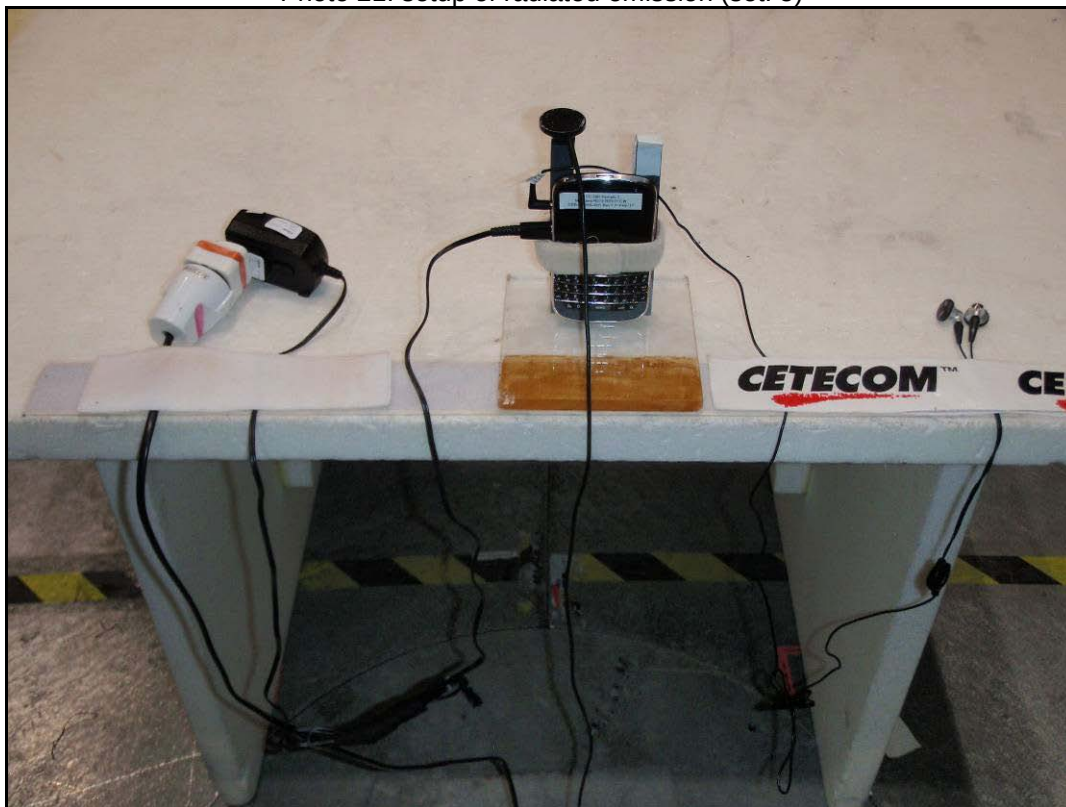
Photo 22: setup of radiated emission (set. 6)
