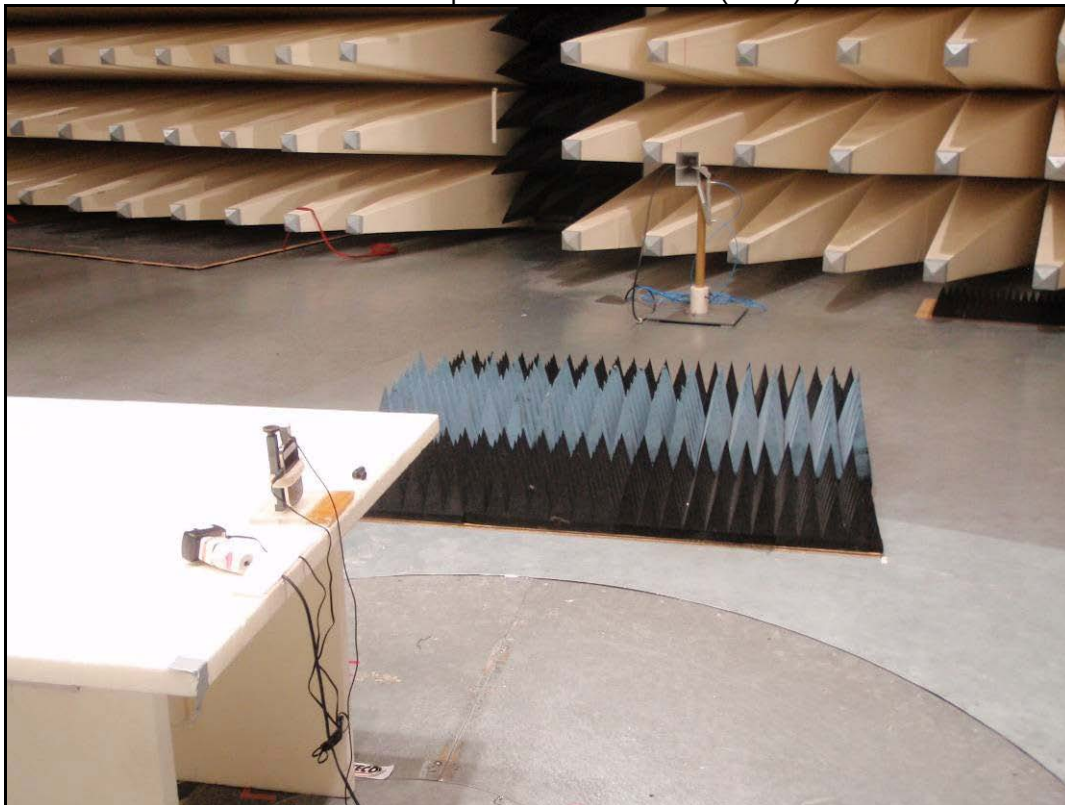
Photo 18: setup of radiated emission (set. 4)
