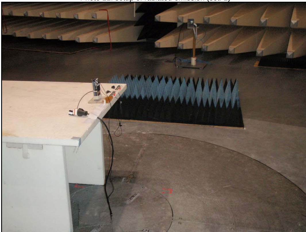
Photo 12: setup of radiated emission (set. 2)
