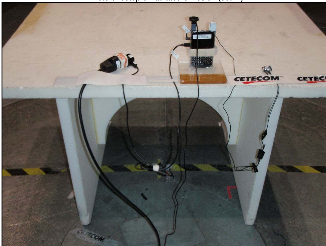
Photo 10: setup of radiated emission (set. 2)
