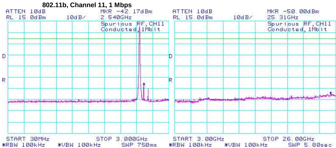
Figure 4-27: Spurious Conducted RF Emissions
