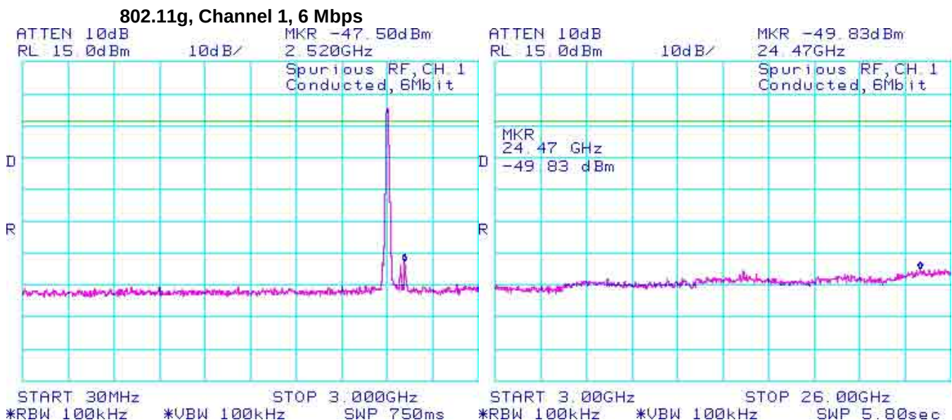
Figure 4-28: Spurious Conducted RF Emissions
