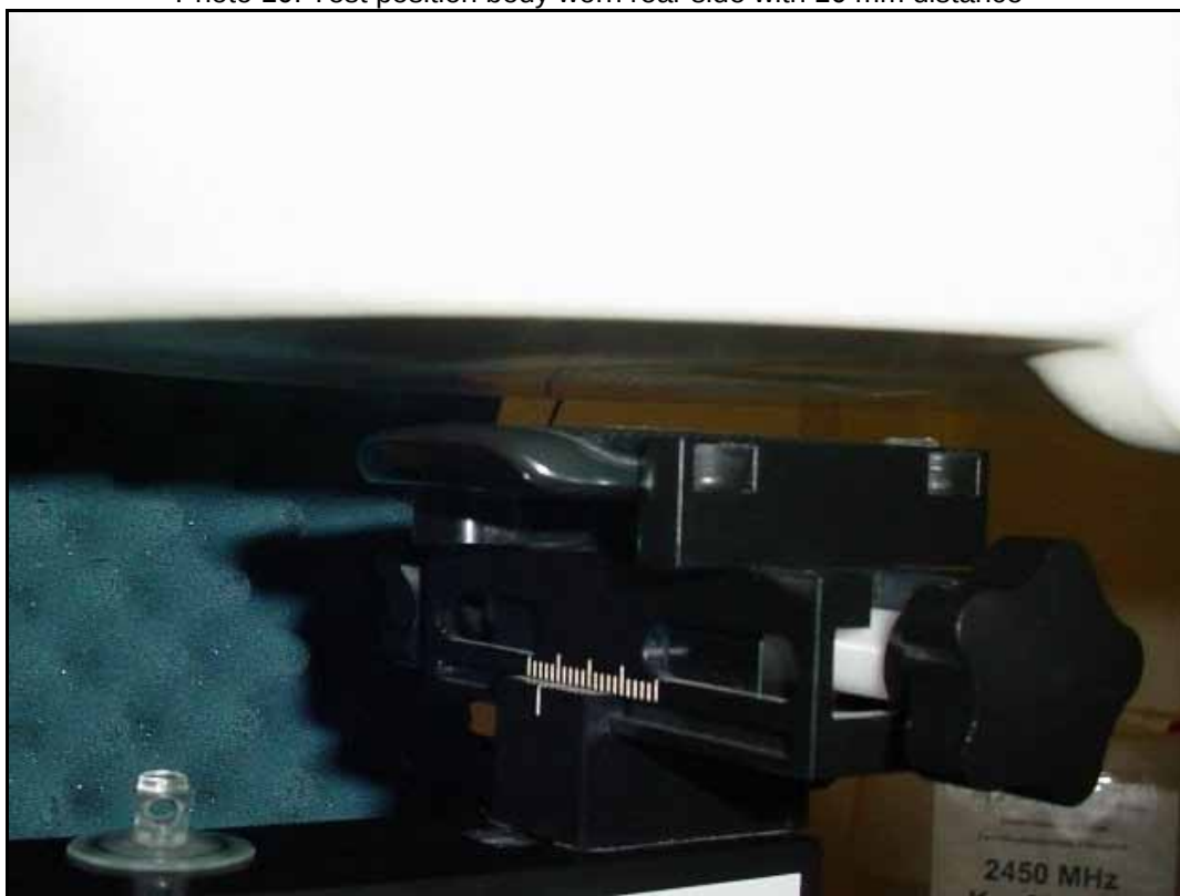
Photo 10: Test position body worn rear side with 10 mm distance
