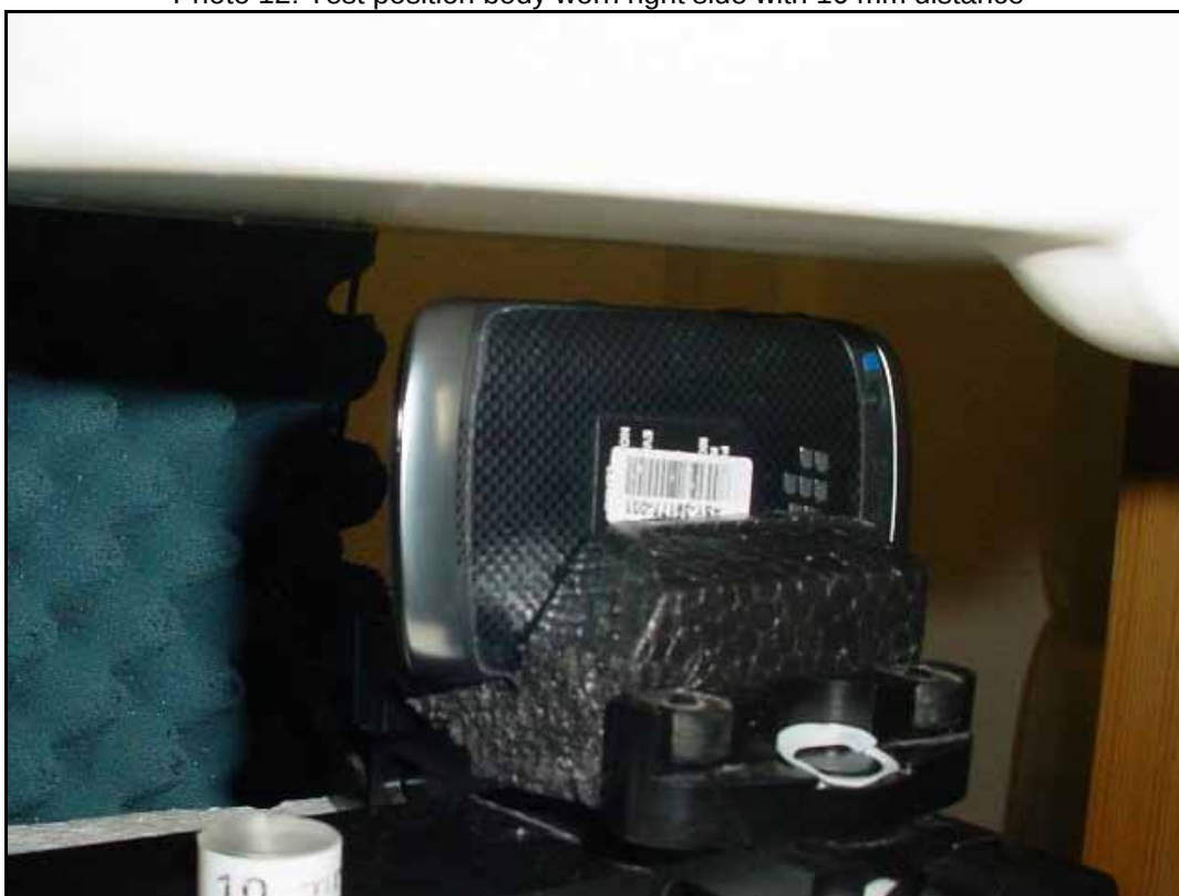
Photo 12: Test position body worn right side with 10 mm distance
