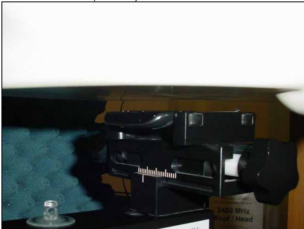
Photo 10: Test position body worn rear side with 10 mm distance
