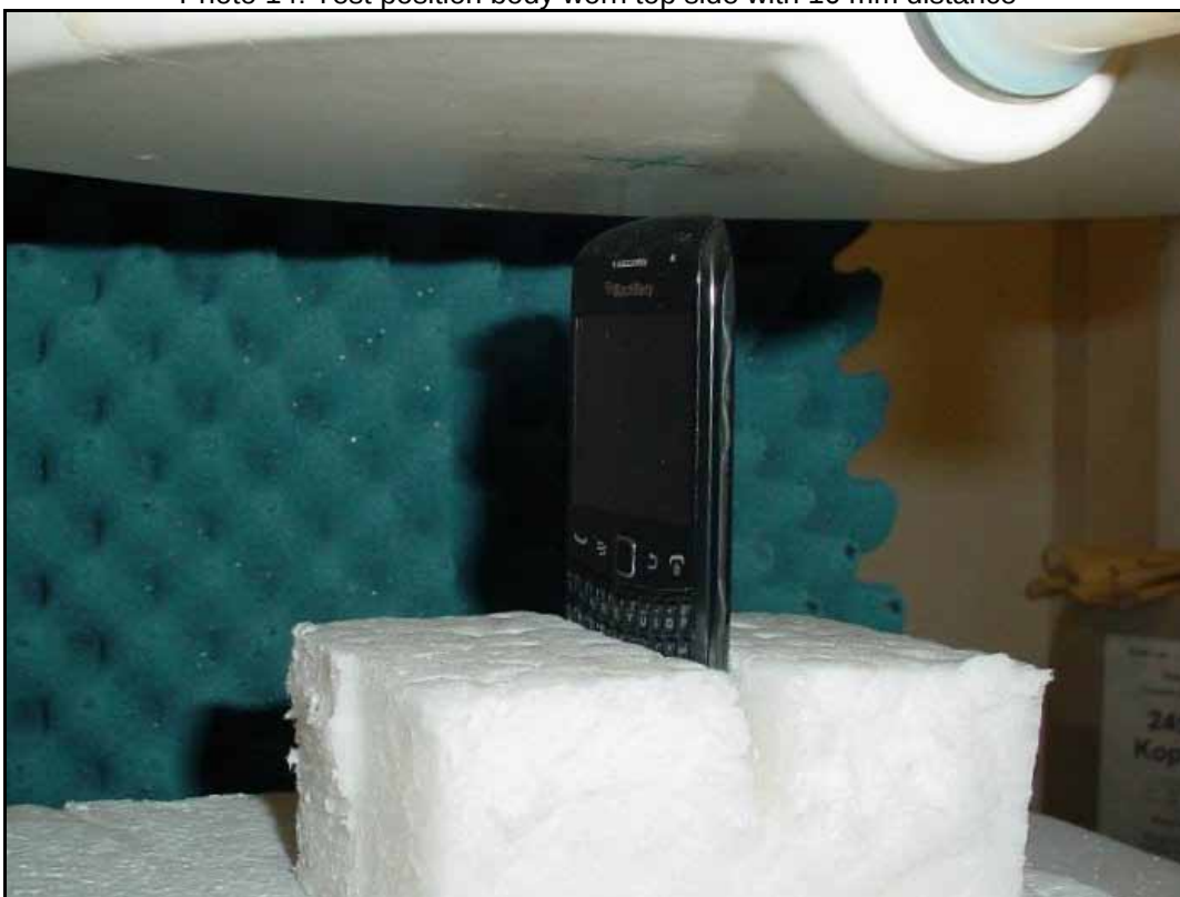
Photo 14: Test position body worn top side with 10 mm distance
