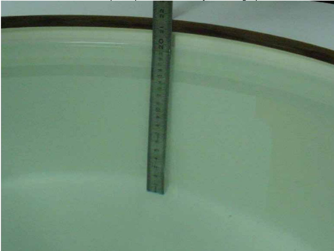
Photo 3: Liquid depth 2450 MHz body simulating liquid
