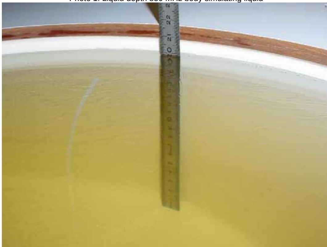
Photo 1: Liquid depth 850 MHz body simulating liquid
