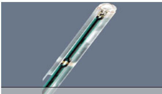
H-Field Probe (H3DV6)
