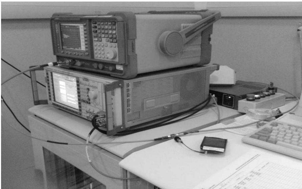
Figure 2 – Dipole Validation & Probe Modulation Factor measurement setup
