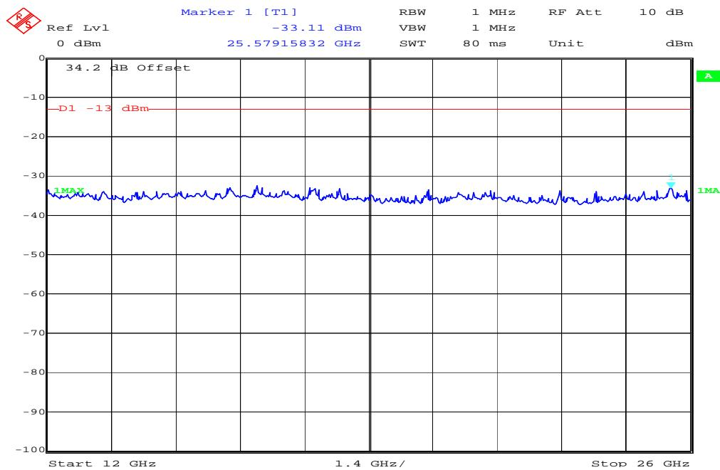
**Channel 512 EDGE (30 MHz – 12GHz) antenna vertical**
