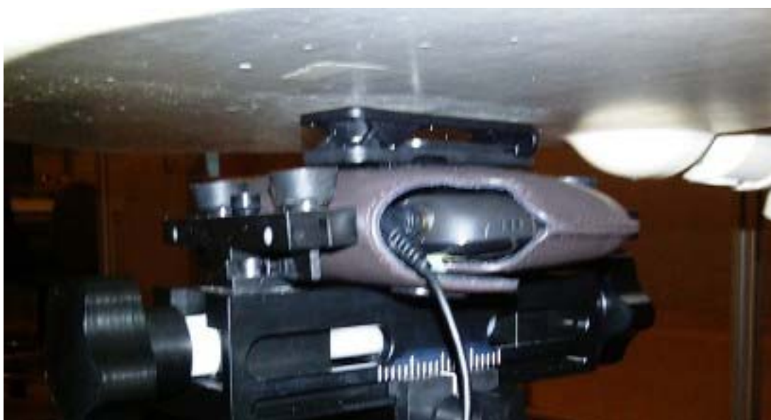
Figure E12. Body-worn configuration (Horizontal Holster, headset 1, back facing phantom)
