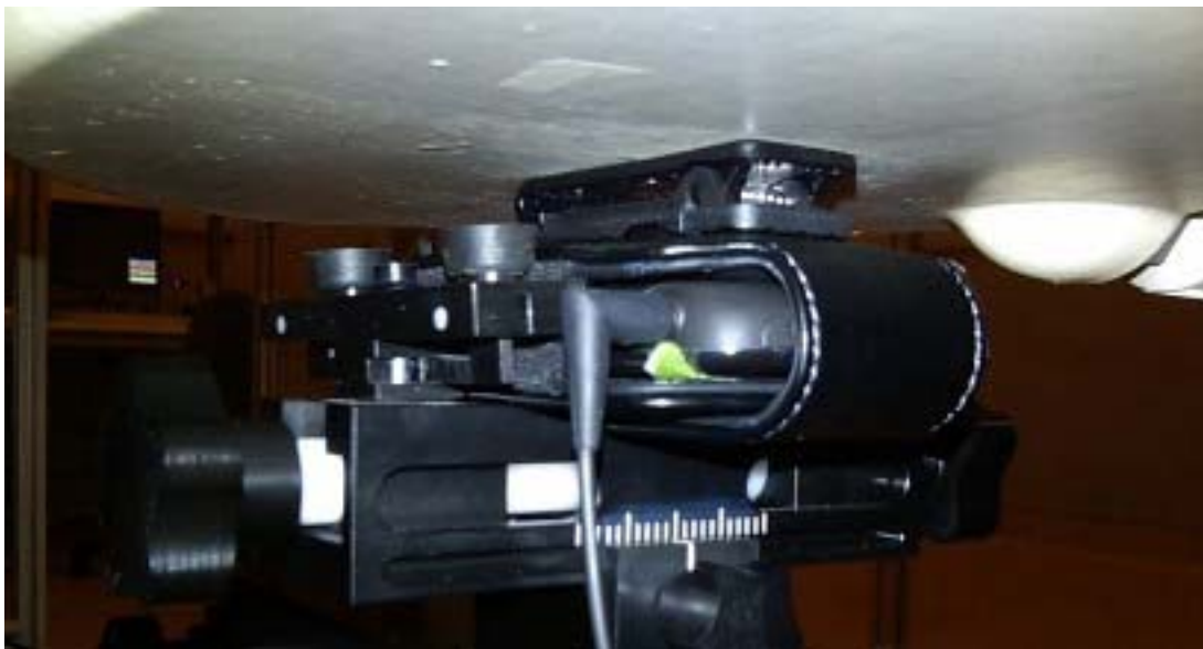
Figure E8. Body-worn configuration (Vertical Holster , headset 2, back facing phantom)
