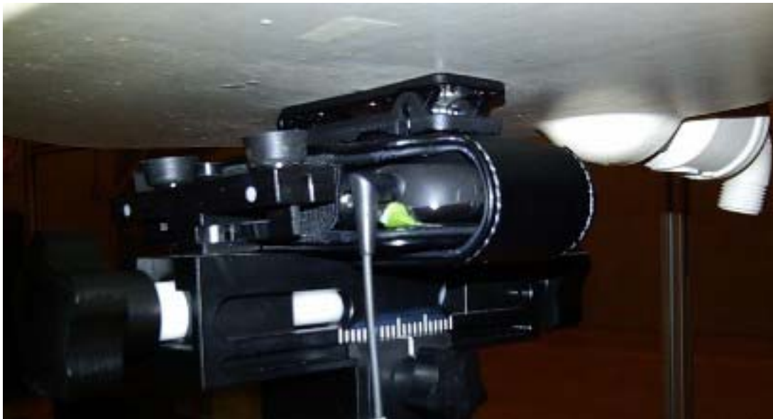
Figure E9. Body-worn configuration (Vertical Holster , headset 3, back facing phantom)
