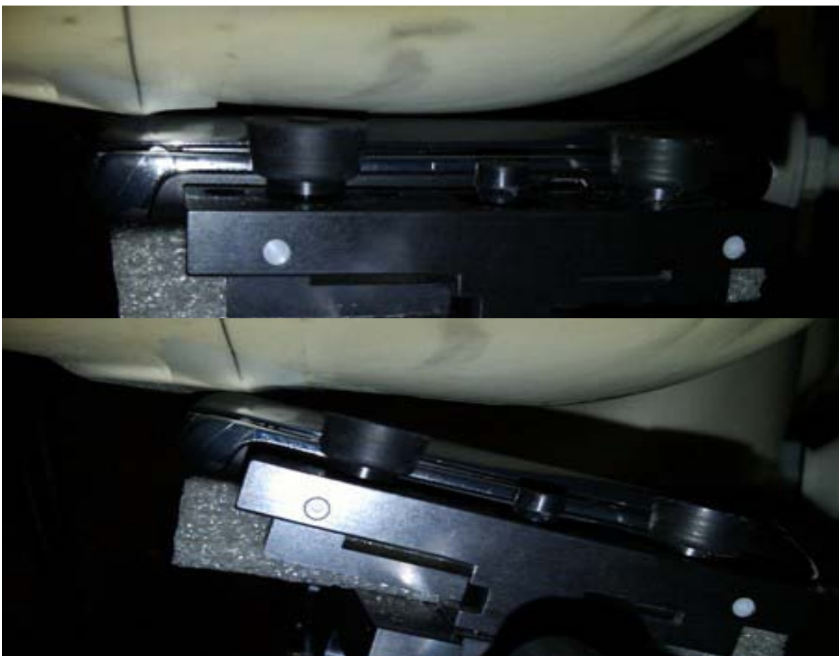
Figure E4. Head configuration (Right Touch/Tilt/Slider Closed)
