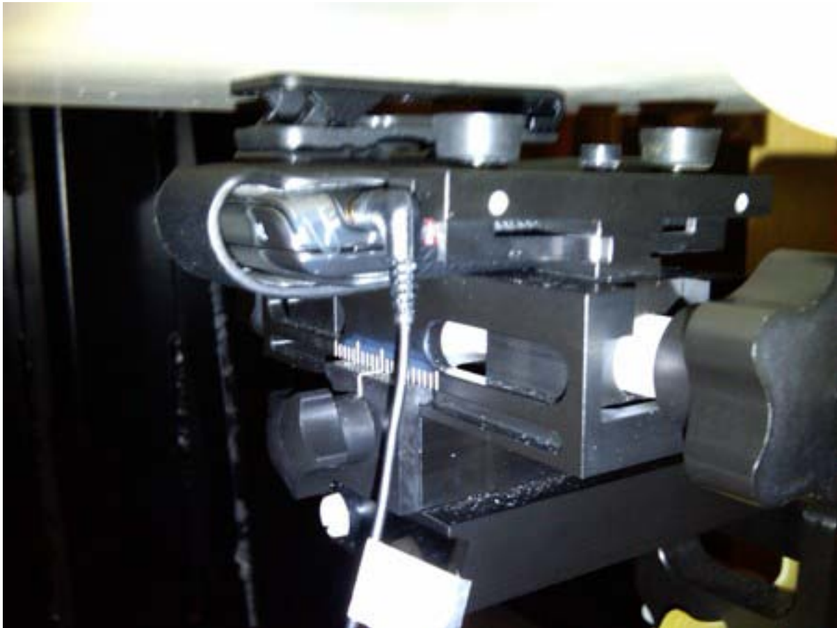
Figure E9. Body-worn configuration (Vertical Holster , headset 1, back facing phantom)
