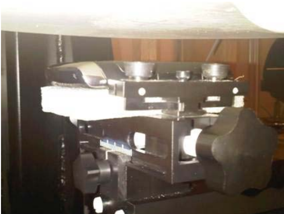
Figure E13. Body-worn configuration (No Holster, 25 mm away, back facing phantom)
