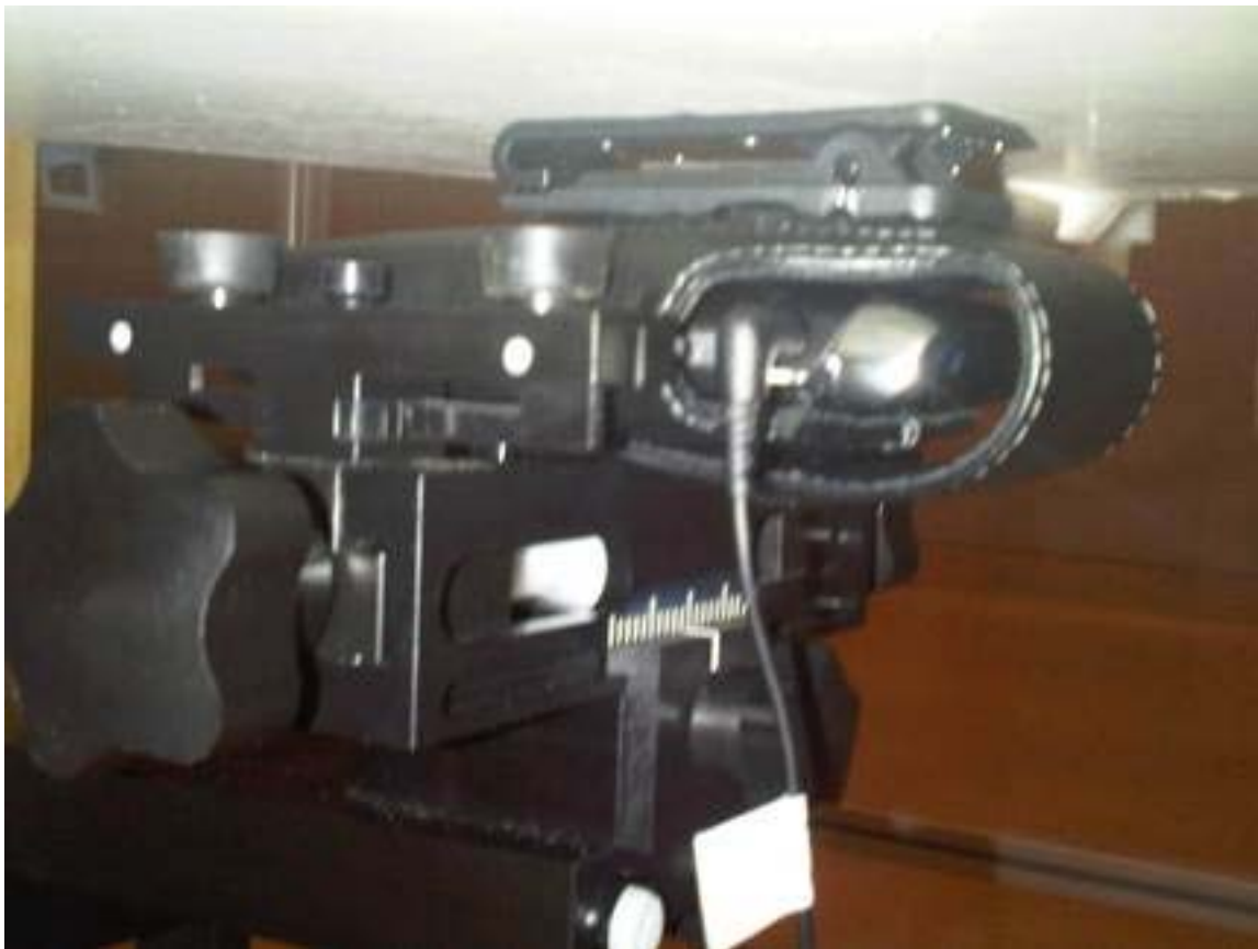
Figure E7. Body-worn configuration (Vertical Holster , headset 1, back facing phantom)
