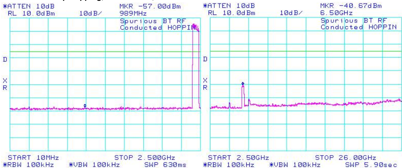
Figure 3-43 : Spurious RF Conducted Emissions
