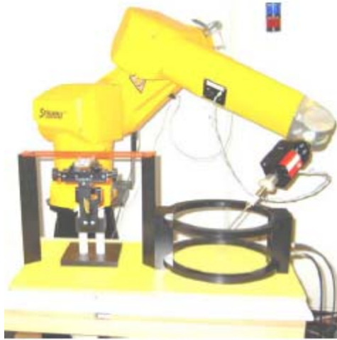
Figure 5.6.1. T-Coil set up with HAC Test Arch with Helmholtz Coil (AMCC)
