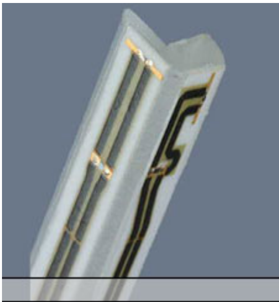
E-Field Probe (ER3DV6)
