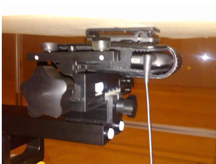
Figure E9. Body-worn configuration (Vertical Holster , headset 3, back facing phantom)
