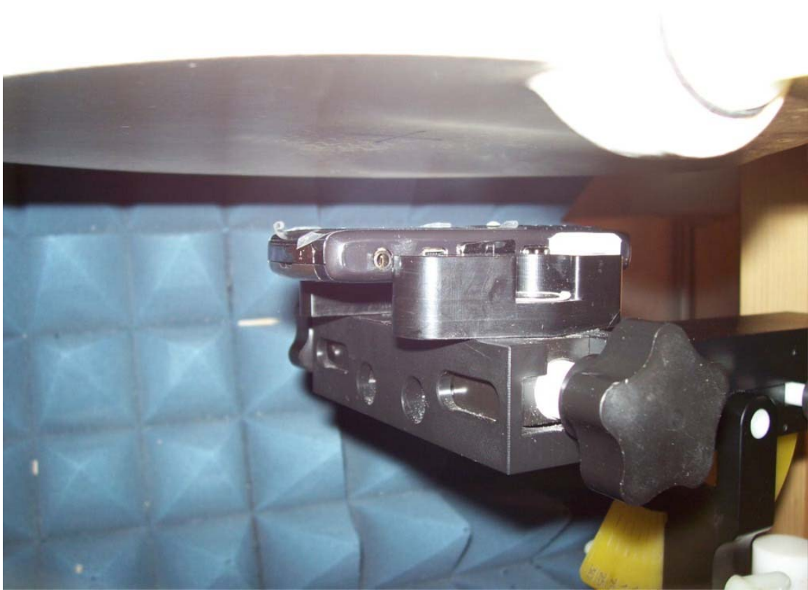
Figure E17. Body-worn configuration (No Holster, 25 mm away, front facing phantom)
