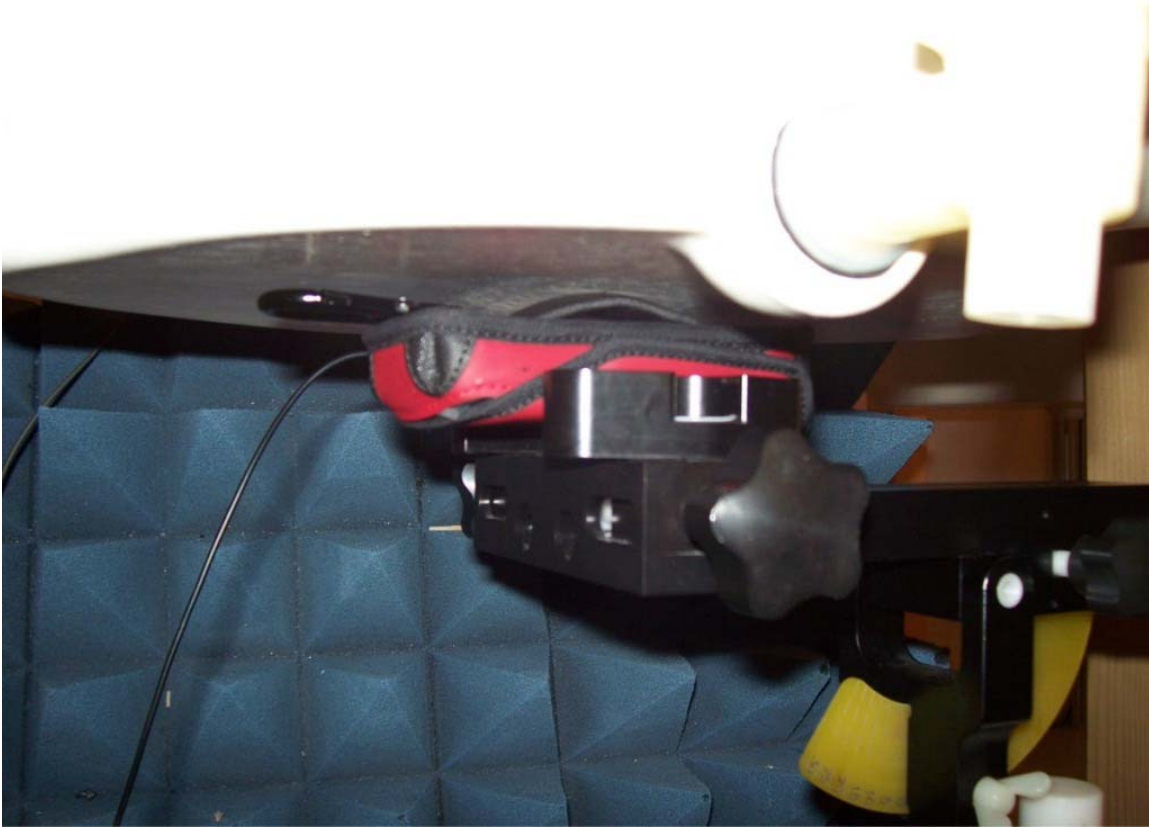
Figure E15. Body-worn configuration (Sportscase with clip, headset, back facing phantom)
