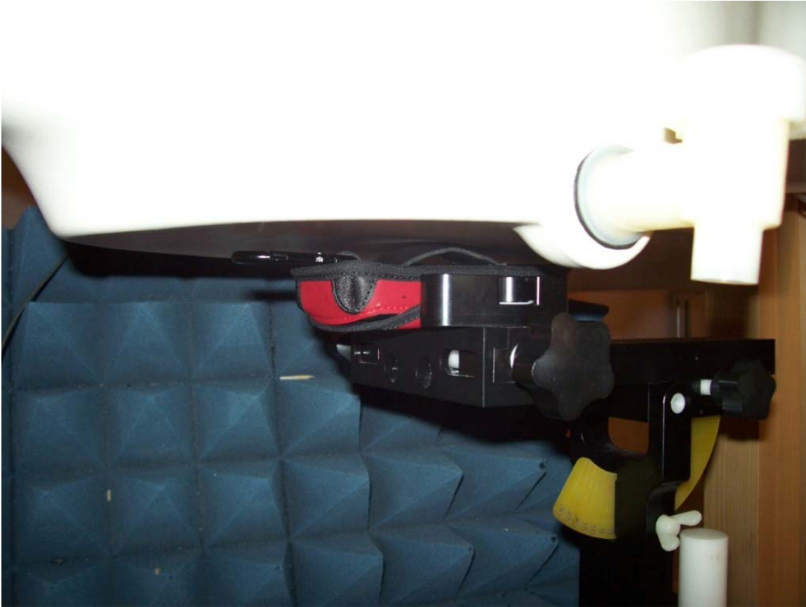
Figure E12. Body-worn configuration (Sportscase with clip, front facing phantom)
