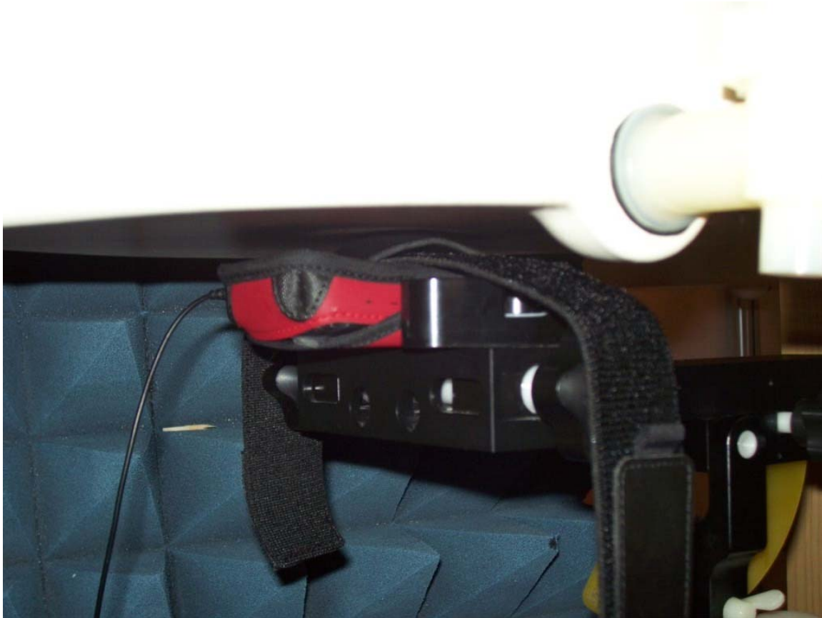
Figure E14. Body-worn configuration (Sportscase with strap, headset, back facing phantom)
