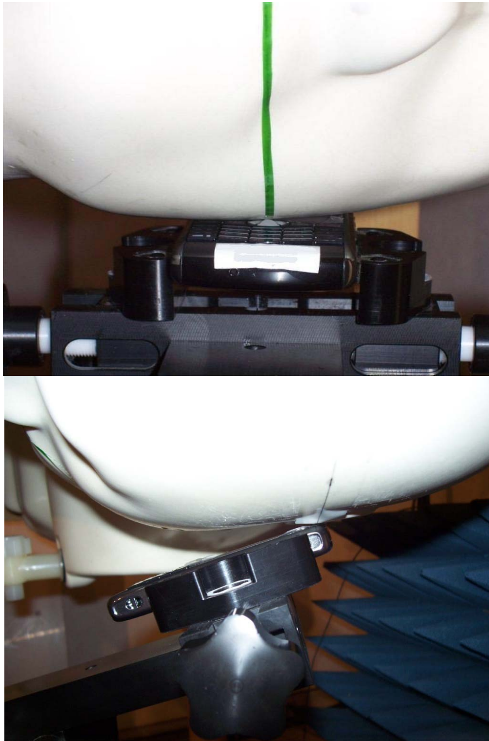
Figure E4. Head configuration (Left Touch/Tilt)
