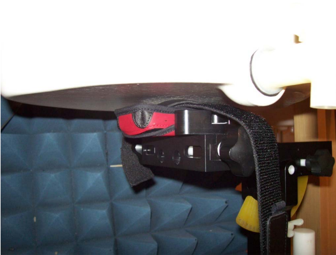
Figure E11. Body-worn configuration (Sportscase with strap, front facing phantom)
