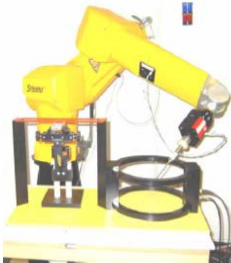
Figure 2: T-Coil set up with HAC Test Arch with Helmholtz Coil (AMCC)
