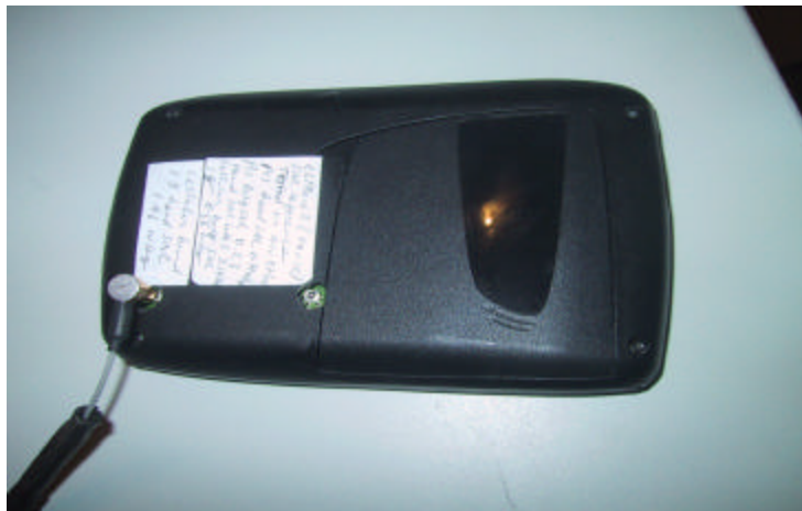
Figure A: Back view of handheld with RF switches and connector for conducted power measurement
