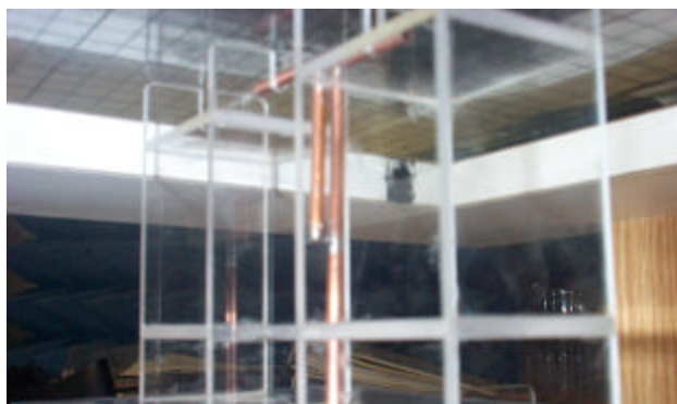
Figure 10. Validation Dipole Under Phantom
