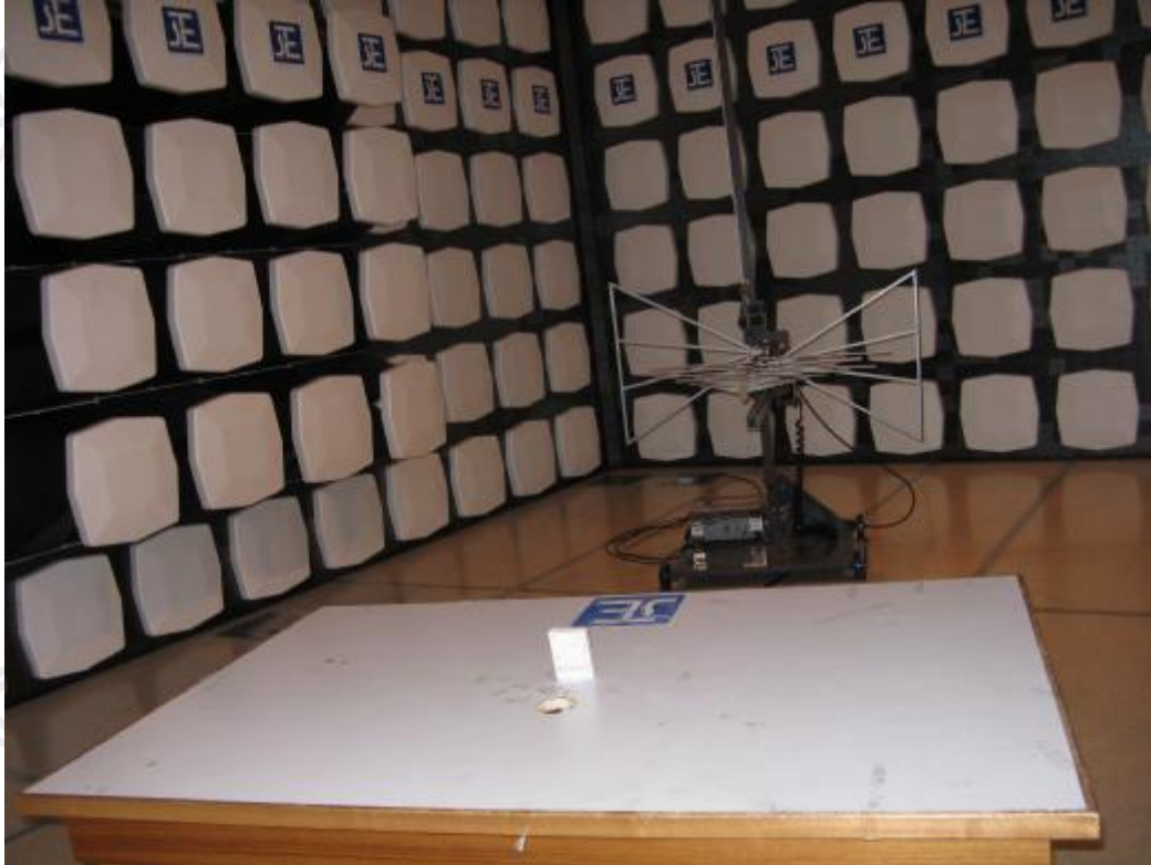
Measurement of Radiated Emission Test Set Up
