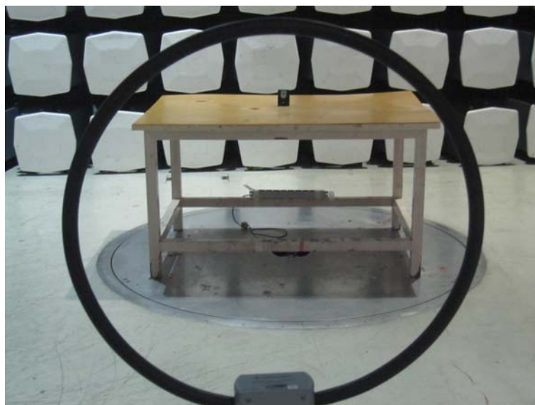
Radiated emission test photo
