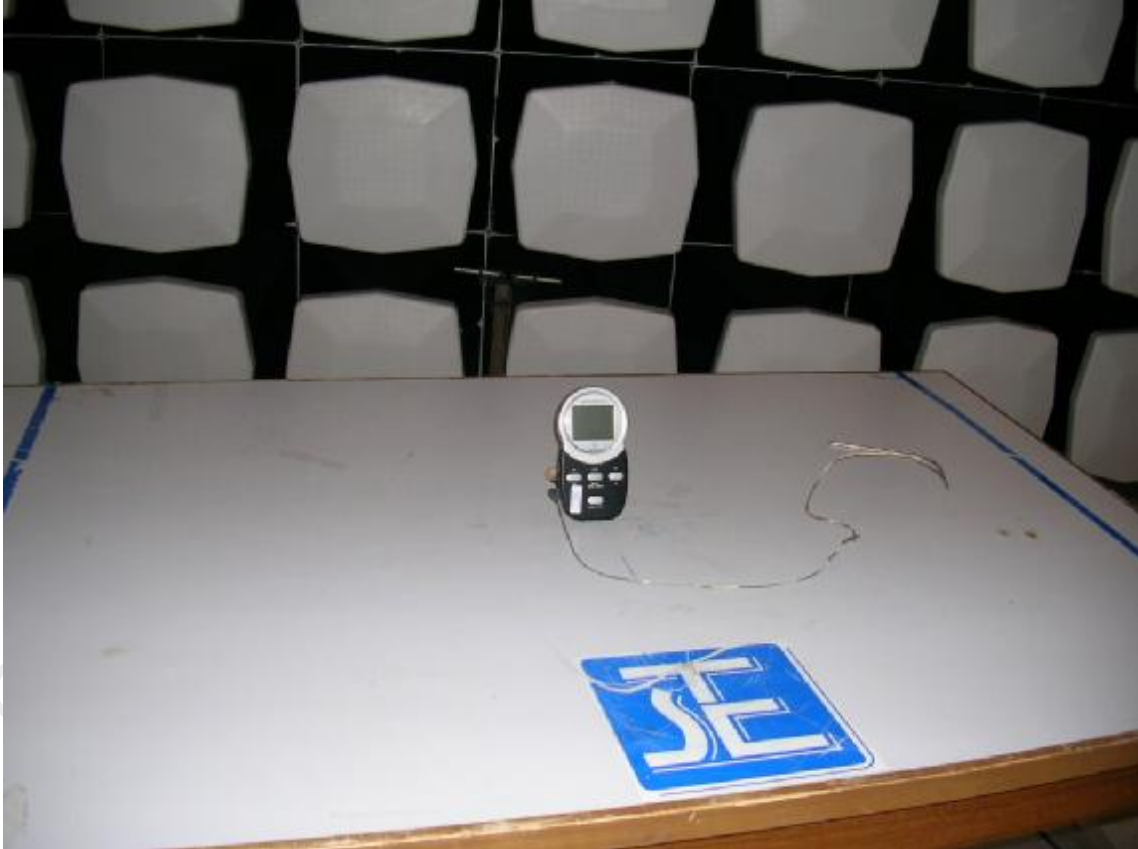
Measurement of Radiated Emission Test Set Up
