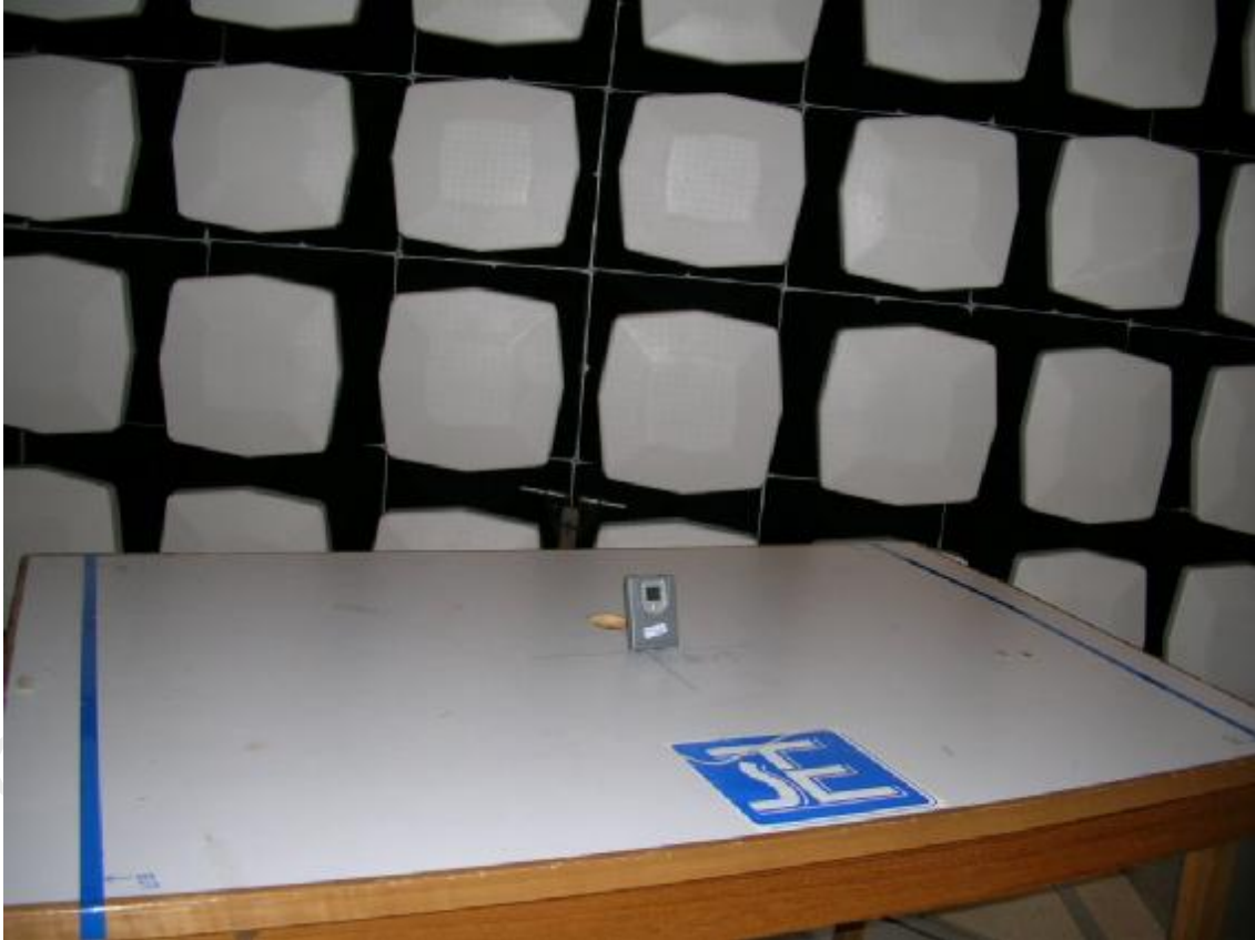
Measurement of Radiated Emission Test Set Up
