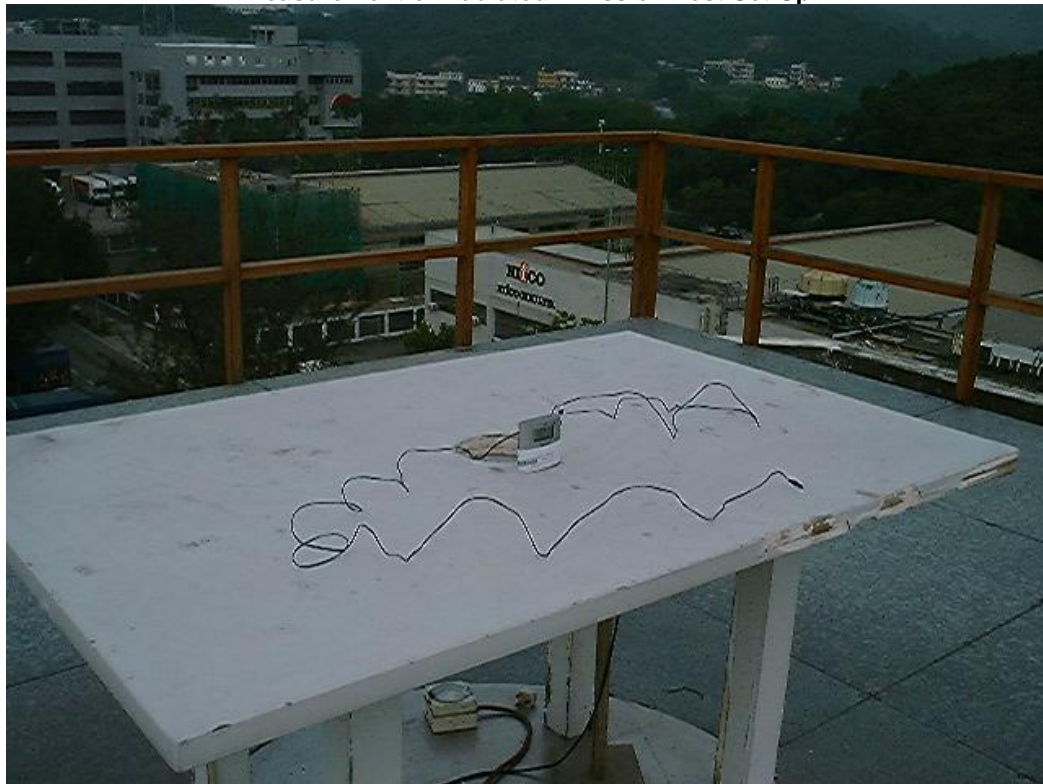
Measurement of Radiated Emission Test Set Up
