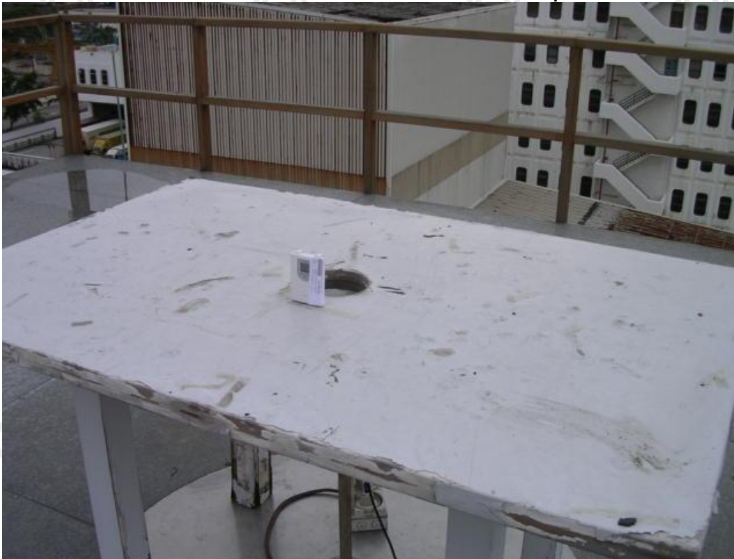
Measurement of Radiated Emission Test Set Up
