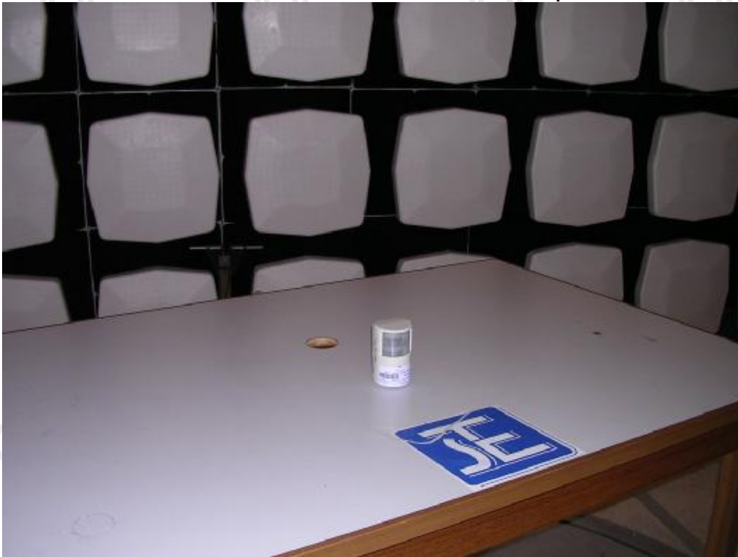
Measurement of Radiated Emission Test Set Up
