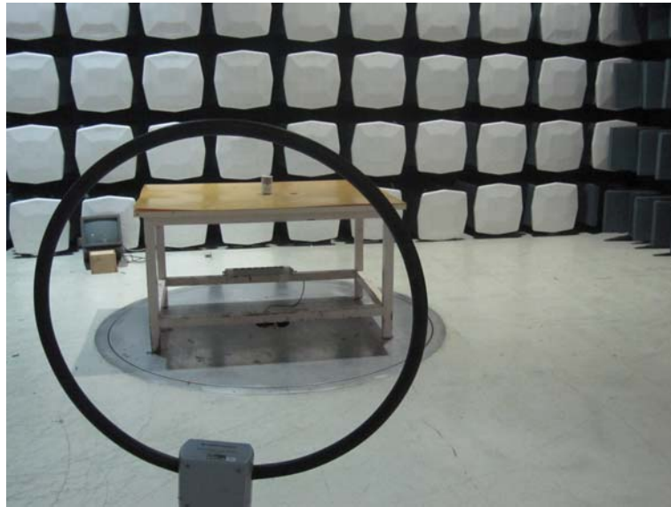
Radiated emission test photo
