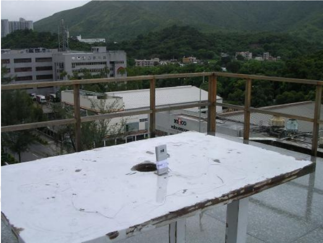
Measurement of Radiated Emission Test Set Up
