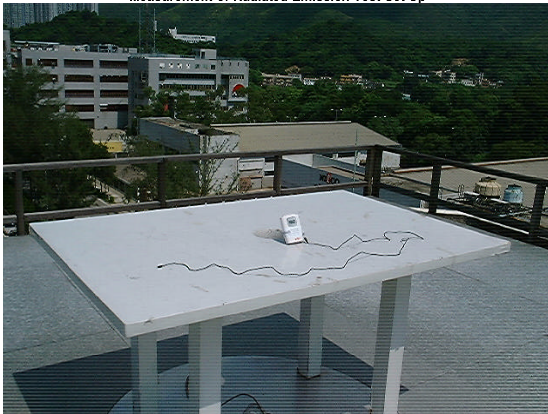
Measurement of Radiated Emission Test Set Up
