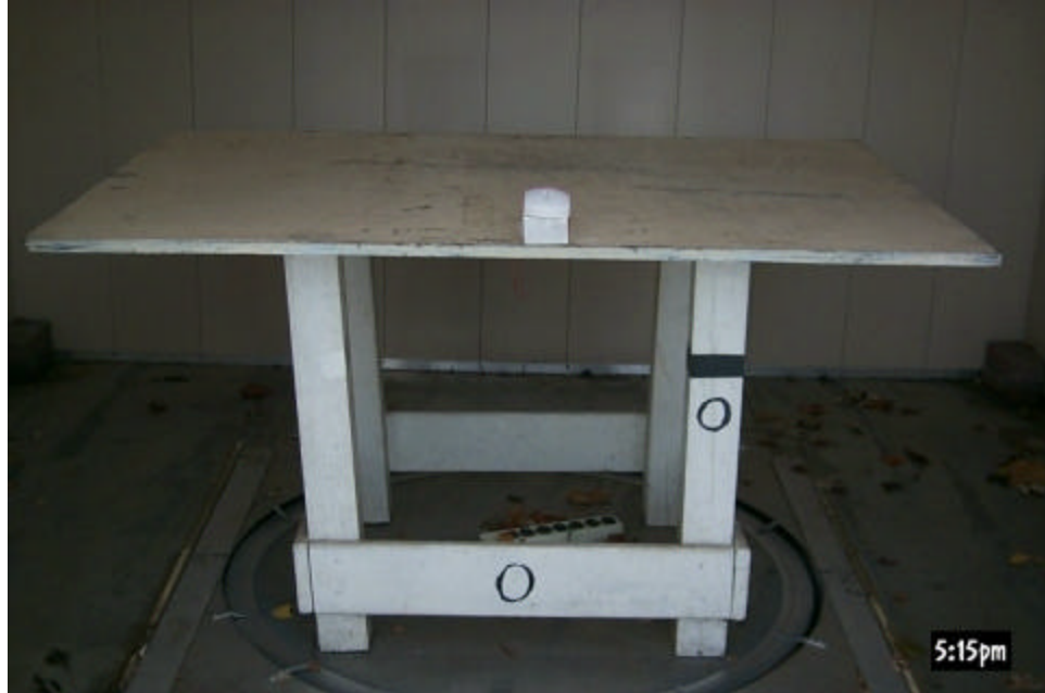
Figure 3.1 Radiated Test Setup, X Axis
