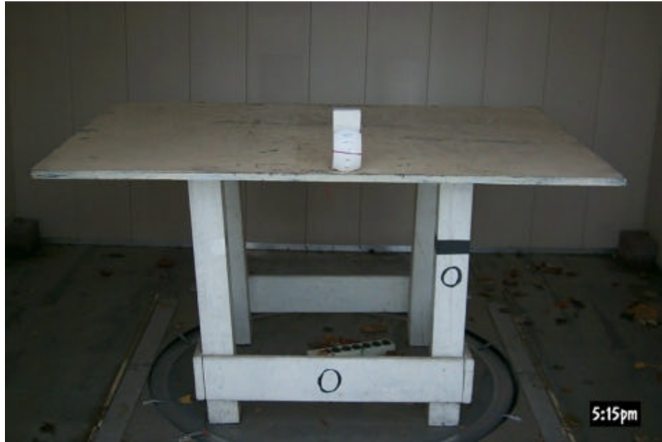
Figure 3.3 Radiated Test Setup, Z Axis
