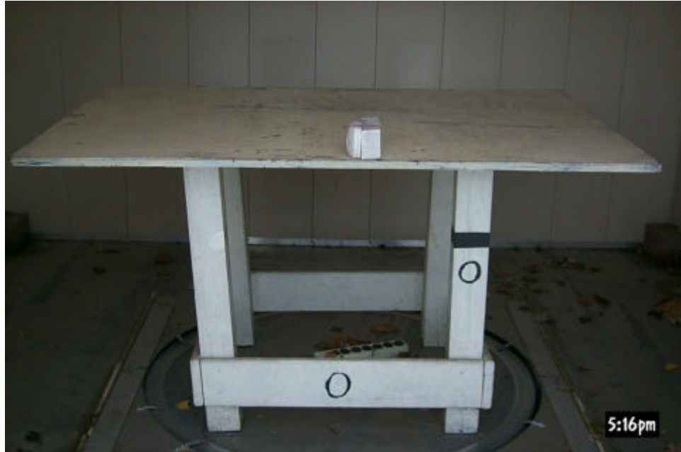
Figure 3.2 Radiated Test Setup, Y Axis
