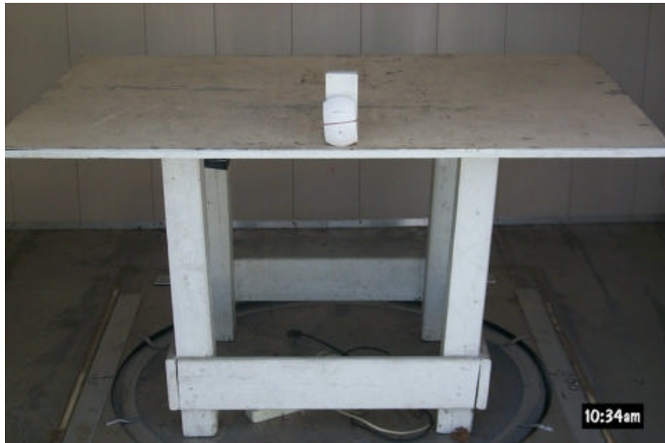
Figure 3.3 Radiated Test Setup, Z Axis
