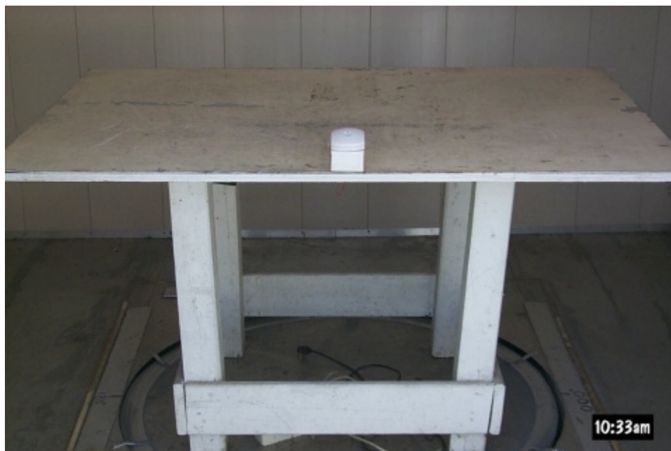
Figure 3.1 Radiated Test Setup, X Axis
