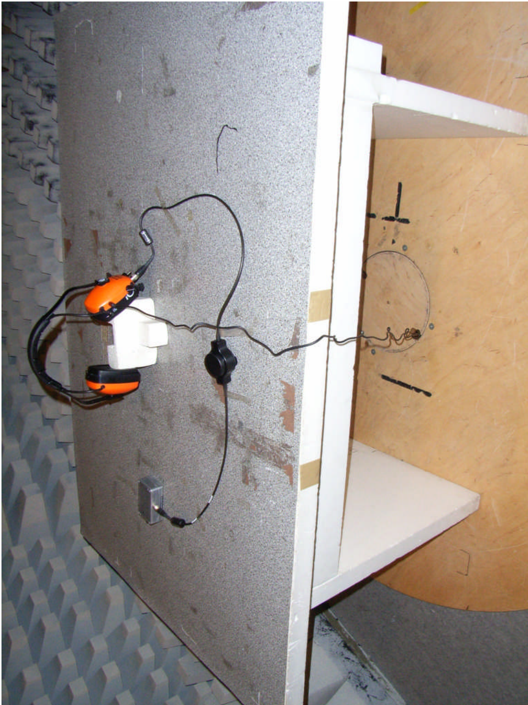
80535_EMI21.jpg Test set-up radiated emission test
