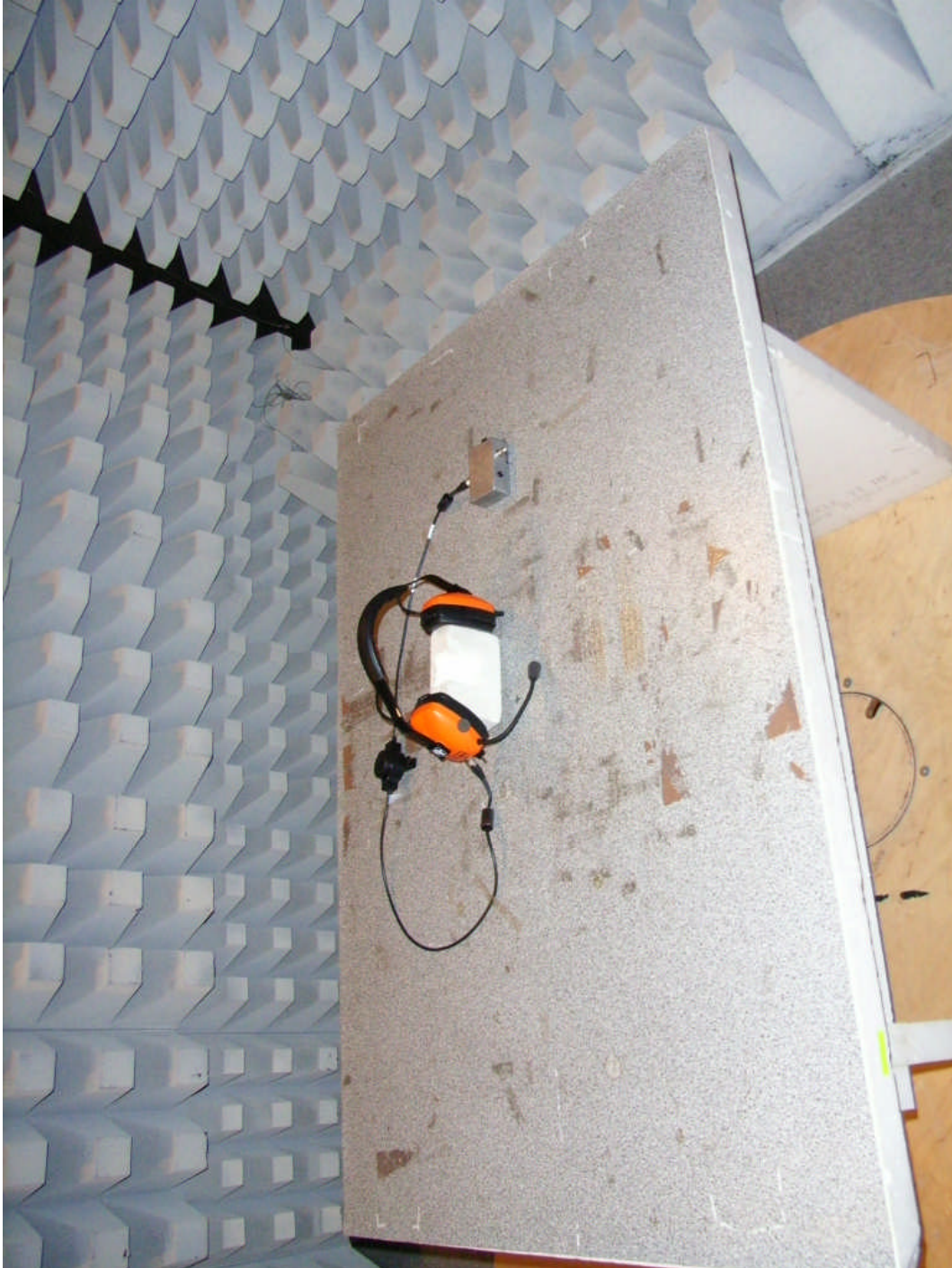
80535_EMI11.jpg Test set-up radiated emission test
