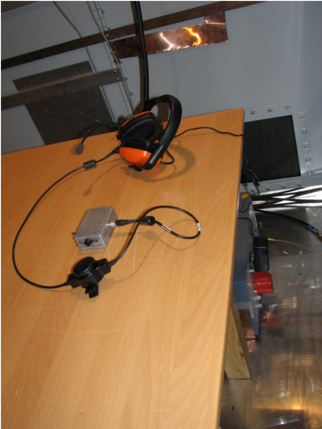
80535_AC10.jpg Test set-up conducted emission
