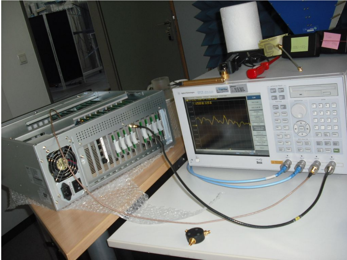
Photo 2: Setup for measurement of the combiner's attenuation
